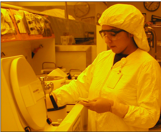
Figure 1. Christine Murabito using a hot plate to do a post-exposure bake during the photolithography process.
