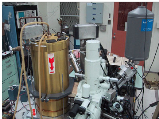
Figure 1. Single-pixel NIST x-ray microcalorimeter system on a scanning-electron microscope. The system was developed in the Electronics and Electrical Engineering Laboratory (EEL) at NIST, Boulder, and transferred to the Chemical Science and Technology Laboratory (CSTL) at NIST Gaithersburg, Maryland to be used to study problems of interest to the semiconductor industry.
