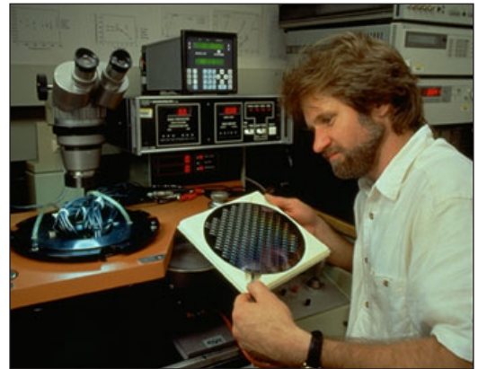
Test wafer being loaded on wafer prober for long-term dielectric testing.
