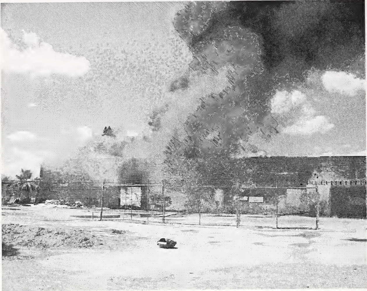
Figure 16. Photograph showing flames through open door and burning roof during the second test.
