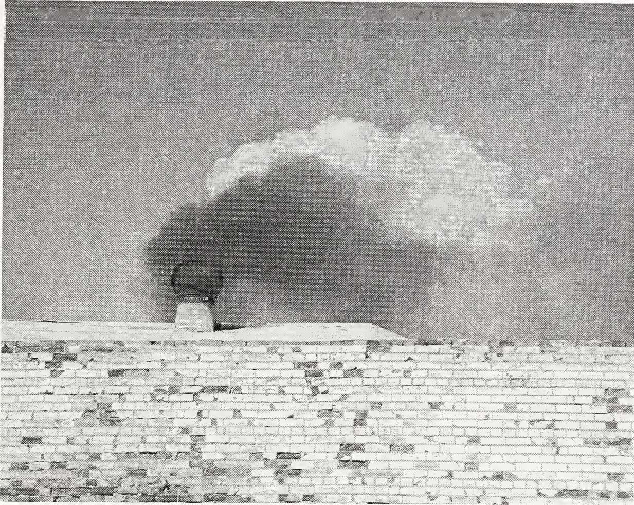
Figure 9. Photograph of smoke coming from roof top ventilator during the first test.
