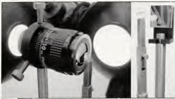
A small beveled mirror placed near the eyepiece of a near-eye display (NED) with an adjustable source to the side can be used to quantify the accuracy of measurement apparatus that claims to be able to measure the light output of NEDs.
