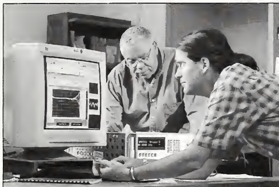
Bryan Waltrip and Robert Palm evaluate the performance of the NIST-developed Wideband Sampling Voltmeter and its associated input probes for making accurate pulse waveform measurements.
