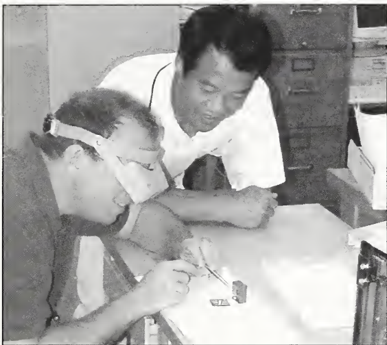
Neil Zimmerman and Yicheng Wang assemble vacuum-gap capacitor prior to cooling to 0.02 K, and testing.
