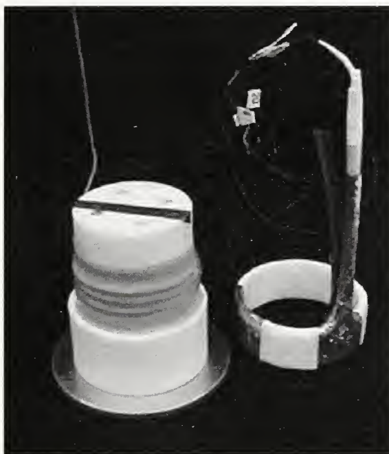
Cryogenic current comparator for measurement of 1 M \Omega directly against the quantum Hall resistance.
