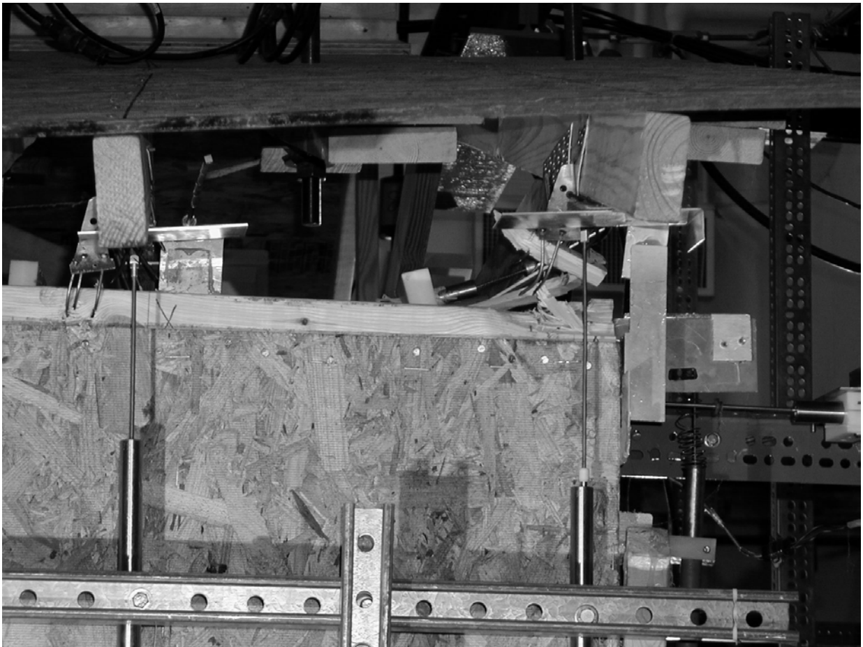
Figure 6.10. Failure of hurricane clip connection with combined load.
