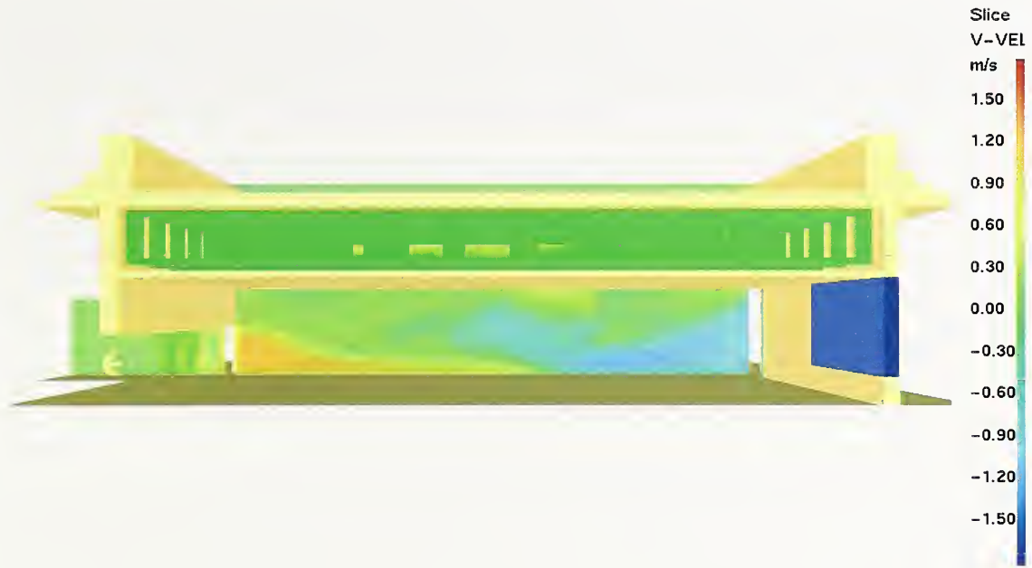
Figure 17. Gas velocities within a vertical plane at 1705 s into the simulation. The double door has been opened on the east side. The blue indicates air moving right to left into the structure.
