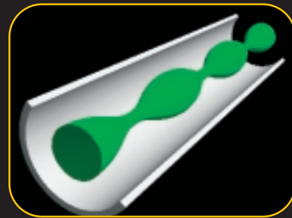
Lattice Boltzmann simulation of the Taylor-Tomotika instability of a fluid thread confined within a tube.
