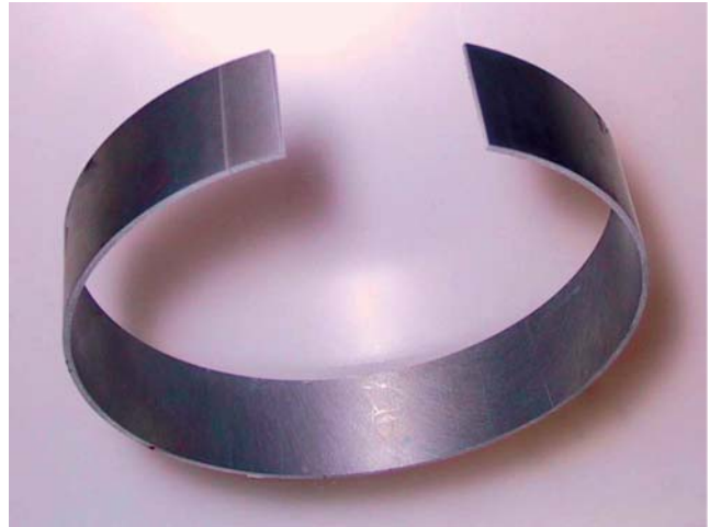
Figure 1: Split ring from Demeri cup springback test.
