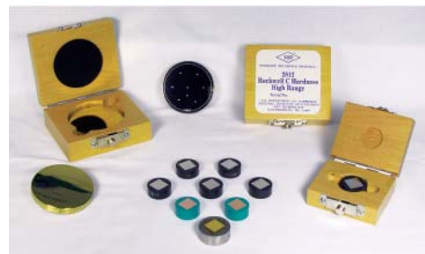
Figure 2: SRM test blocks for Rockwell, Vickers and Knoop hardness (metals).
