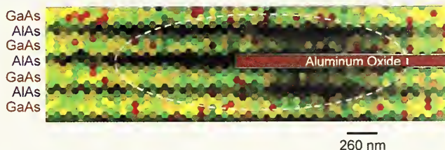
Figure 1: Crystallographic orientation map with darker pixels indicating greater pattern diffuseness or strain.
