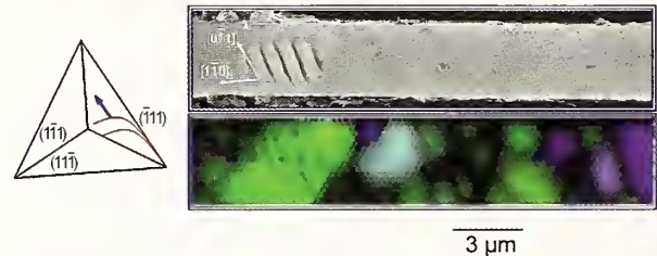
Figure 1: Dislocation mechanism for topography formation induced by AC stressing in Al-1Si.
