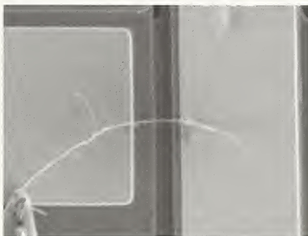
Figure 4: SEM image of attaching a nanotube to a MEMS device, in progress. Development of carbon deposits can be seen near the edges of the MEMS under the nanotube. The nanotube rope is about 100 nm in diameter. The tip of the tungsten probe that maneuvers the nanotube can be seen in the lower left corner of the image.
