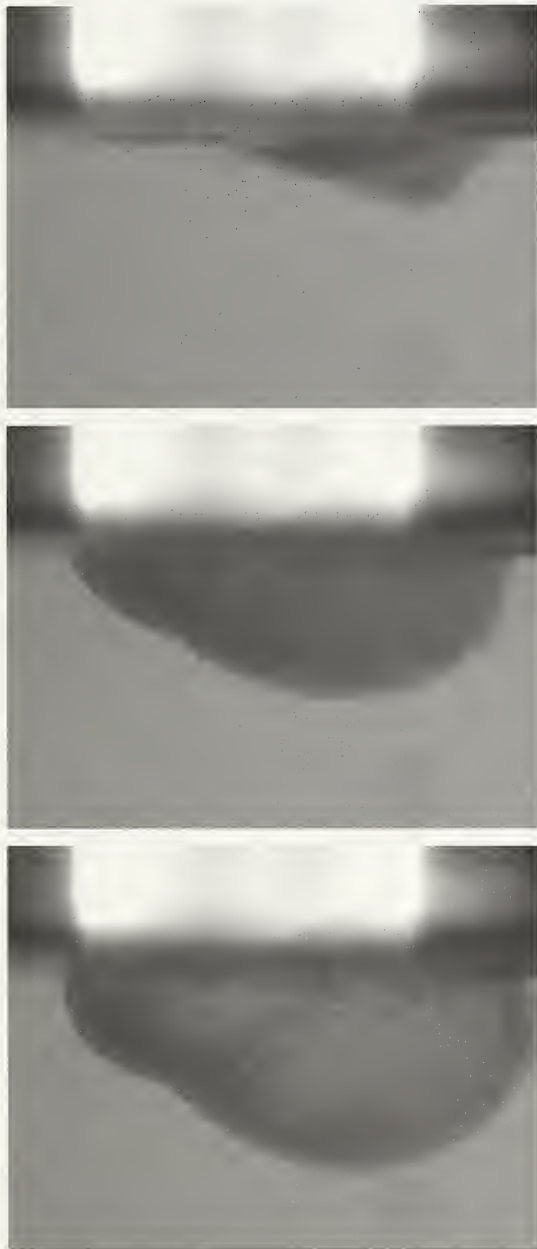
Figure 1: Images of a rat pulmonary artery at the start of the biaxial test, at ~2 psi, and at ~4 psi. Field width = 4 mm.
