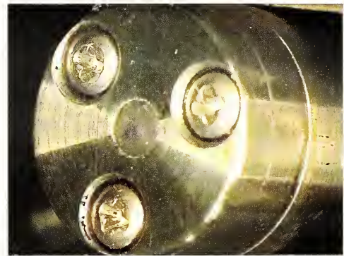
Figure 1: Biaxial test fixture developed at NIST. The tissue is tested by pressurizing the backside of the 3 mm diameter gauge section located at the center.
