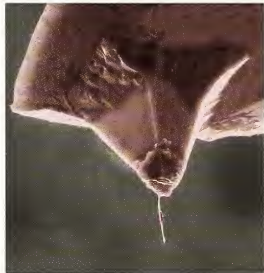
Figure 1: SEM micrograph of carbon nanotubes attached to the end of an AFM tip. The long slender tip is 100 nm in diameter and is made of several multiwalled nanotubes wound together similar to a rope.
