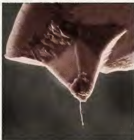
Figure 2: Scanning electron microscope (SEM) image of nanotube attached to an AFM tip with applied adhesive. The nanotube is actually a rope of several tubes about 100 nm in diameter.
