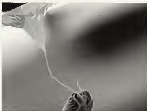
Figure 3: SEM image of tungsten probe (bottom of image) attaching a 20 mm long nanotube rope to the end of an AFM tip (upper left) using EBD. After this nanotube rope was attached, it was pulled until the tube separated from the tungsten probe.
