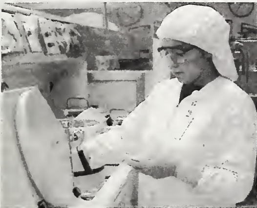
Figure 1. Christine Murabito using hot plate to do a post-exposure bake during the photo-lithography process.
