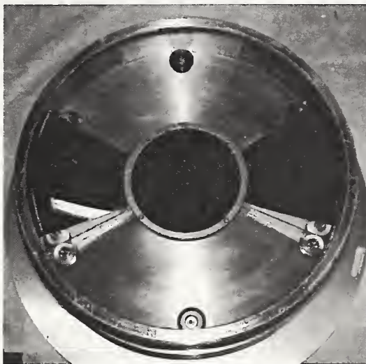
Figure 1. C-1 Mirror from the ETS of the EUV-LLC. Only two of the six sectors are shown. The laser-plasma source is positioned on the central axis.
