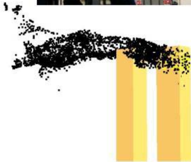
Figure 4: Comparison of a photograph ( ©2001 Kevin Ready. All rights reserved. Used by permission.) and of a frame from simulation of the WTC tower fires, showing the quasisteady smoke plume generated by the fire in the north tower.
