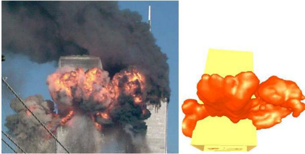
Figure 6: Comparison of a photograph ( ©2001 Sara K. Schwittek. All rights reserved. Used by permission.) and a simulation image of the south tower fireball shortly after the collision with the second hijacked plane.
