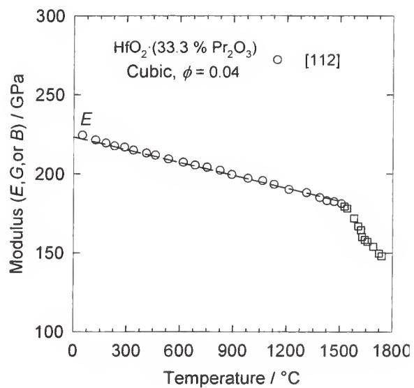
$\text{HfO}_2 \cdot x\text{Pr}_2\text{O}_3$  (cubic) { hafnium oxide, hafnia,  $\text{Pr}\text{-}\text{HfO}_2(\text{c})$ , praseodymia stabilized cubic hafnia }
