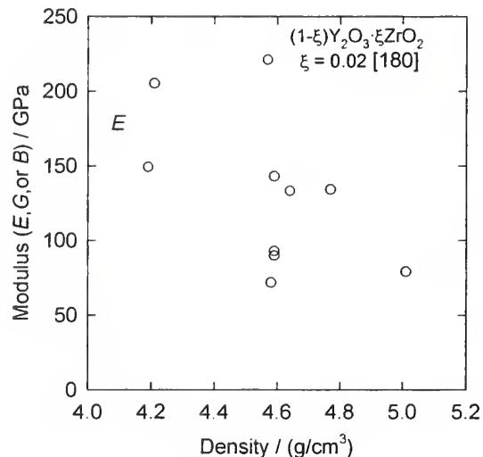
$\text{Y}_2\text{O}_3 \cdot x\text{ZrO}_2$  (yttria, Zr-Y<sub>2</sub>O<sub>3</sub>, zirconia-doped yttria)
