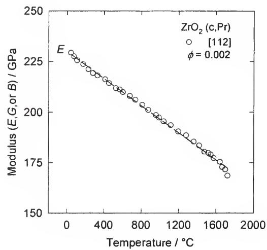
**ZrO<sub>2</sub> · xPr<sub>2</sub>O<sub>3</sub> (cubic) { zirconium dioxide, zirconia, Pr-ZrO<sub>2</sub>(c), Pr-stabilized cubic zirconia }**
