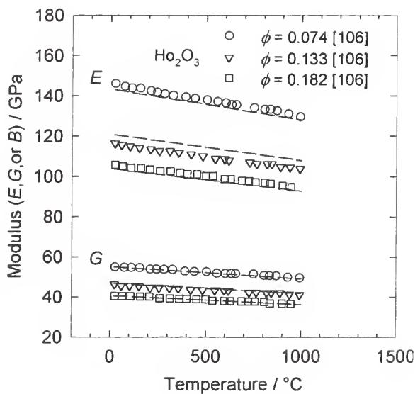
**Ho<sub>2</sub>O<sub>3</sub> { holmium oxide, holmia }**
