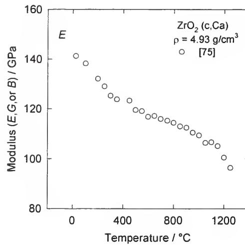
$\text{ZrO}_2 \cdot x\text{CaO}$  (cubic) { zirconium dioxide, zirconia,  $\text{Ca-ZrO}_2(\text{c})$ , Ca-stabilized cubic zirconia }
