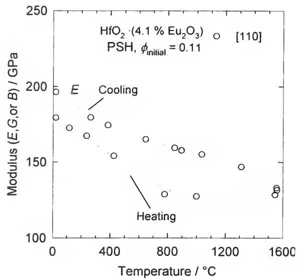
$\text{HfO}_2 \cdot x\text{Eu}_2\text{O}_3$  (partially stabilized) { hafnium oxide, hafnia, Eu-PSH, europia partially stabilized hafnia }
