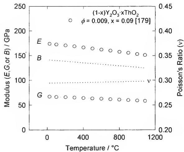
$\text{Y}_2\text{O}_3 \cdot x\text{ThO}_2$  { yttria, Th-Y<sub>2</sub>O<sub>3</sub>, thorium-doped yttria }
