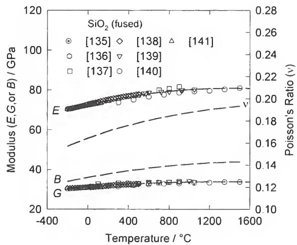
**SiO<sub>2</sub> { silicon dioxide; silica, fused silica, fused quartz, vitreous silica }**
