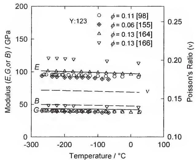
**YBa<sub>2</sub>Cu<sub>3</sub>O<sub>7-x</sub> { yttrium barium copper oxide, Y:123, YBCO }**
