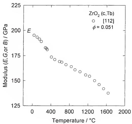
$\text{ZrO}_2 \cdot x\text{Tb}_2\text{O}_3$  (cubic) { zirconium dioxide, zirconia,  $\text{Tb-ZrO}_2(\text{c})$ , Tb-stabilized cubic zirconia }
