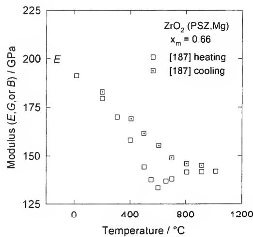
$ZrO_2 \cdot xMgO$  (partially stabilized) { zirconium dioxide, zirconia, Mg-PSZ, magnesia partially stabilized zirconia }
