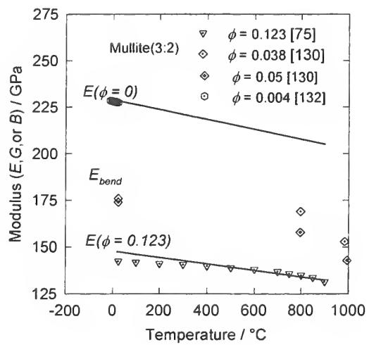
**Al<sub>6</sub>Si<sub>2</sub>O<sub>13</sub> { mullite, mullite(3:2), 3Al<sub>2</sub>O<sub>3</sub> · 2SiO<sub>2</sub> }**
