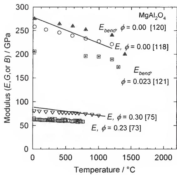
**MgAl<sub>2</sub>O<sub>4</sub> { magnesium aluminate (spinel) }**
