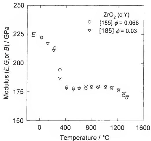
$\text{ZrO}_2 \cdot x\text{Y}_2\text{O}_3$  { zirconium dioxide, zirconia, Y-ZrO<sub>2</sub>(c), Y-stabilized cubic zirconia }
