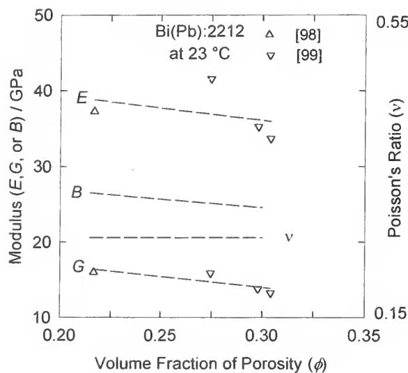
**Bi<sub>2-x</sub>Pb<sub>x</sub>Sr<sub>2</sub>CaCu<sub>2</sub>O<sub>8+y</sub> { Bi(Pb)-2212 }**
