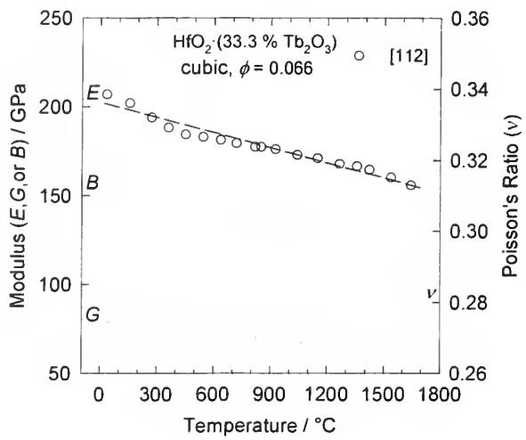
$\text{HfO}_2 \cdot x\text{Tb}_2\text{O}_3$  { hafnium oxide, hafnia, Tb-HfO<sub>2</sub>(c), terbia stabilized cubic hafnia }
