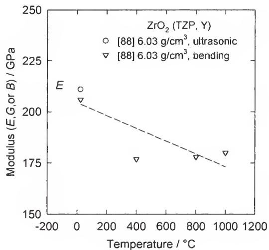
$\text{ZrO}_2 \cdot x\text{Y}_2\text{O}_3$  (tetragonal) { zirconium dioxide, zirconia, Y-TZP, yttria stabilized tetragonal zirconia polycrystal }
