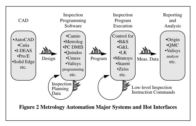
The CAD system of Figure 2 has the same function as the CAD module of Figure 1. A solid modeler is assumed to be part of the CAD system.
