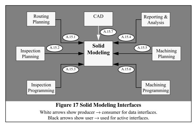
A solid modeler may be needed by CAD, Inspection Planning, Inspection Programming, Machining Planning, Machining Programming, and Routing Planning. Solid Modeling is performed by a solid modeler. Solid modelers are large, complex programs available from only a handful of vendors. Hundreds of person-years are required to build a good one. The best-known solid modelers are ACIS and Parasolid.
