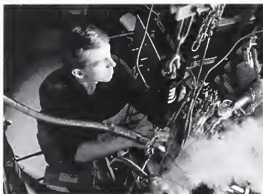
NRC Postdoc Bill Huber preparing for measurements on SET devices at temperatures near 30 mK.
