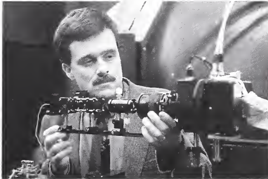
Paul Boynton makes adjustments on an instrument to measure the scattering properties of candidate liquids to be used with the simulated-eye-design camera.
