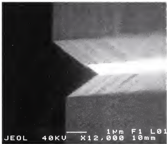
Micrograph of triangle etched in Si: this picture was taken at a tilt of 80°; the black area to the left is the cleaved edge of the Si wafer. Note that, over tens of microns, the triangle has basically no deviations in shape or size.
