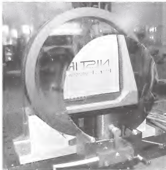
CURRENT WAFER HOLDING MECHANISM (VIEWED FROM THE WAFER BACK SIDE). THE SMALL VACUUM ORIFICE IS SEEN AT THE LOWER EDGE OF THE 200 MM WAFER. BEYOND THE WAFER IS AN F/6 300 MM COLLIMATOR.
