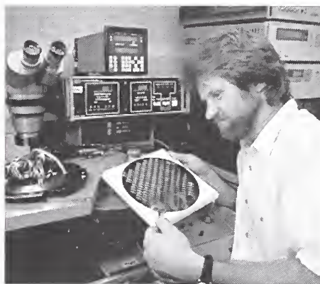
TEST WAFER BEING LOADED ON WAFER PROBER FOR LONG-TERM DIELECTRIC TESTING.
