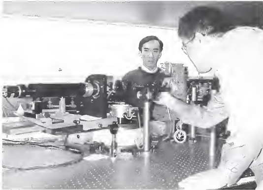
Nhan Van Nguyen (left) and Yong Cho (right) aligning sample on custom-built high-accuracy spectroscopic ellipsometer.
