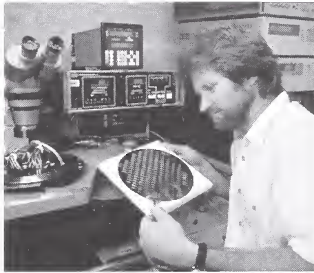
John Suehle loading a test wafer on a wafer prober for long-term dielectric testing.
