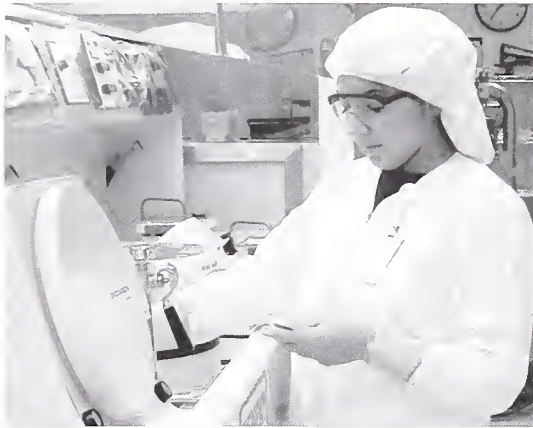
Christine Murabito using a hot plate to do a post-exposure bake during the photo-lithography process.
