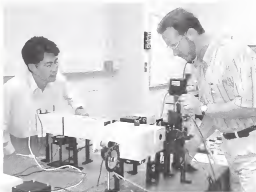
Young-Ho Buh (left) and Glen Birdwell (right) loading a sample onto the stage of the modulation/surface photovoltage spectroscopy system.
