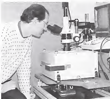
Richard Allen aligning probe card to silicon substrate under test.
