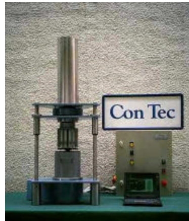
Figure 2: The ConTec viscometers: a) Version 3; b) Version 4.
