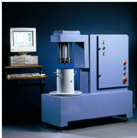
Figure 2: The ConTec viscometers: a) Version 3; b) Version 4.
