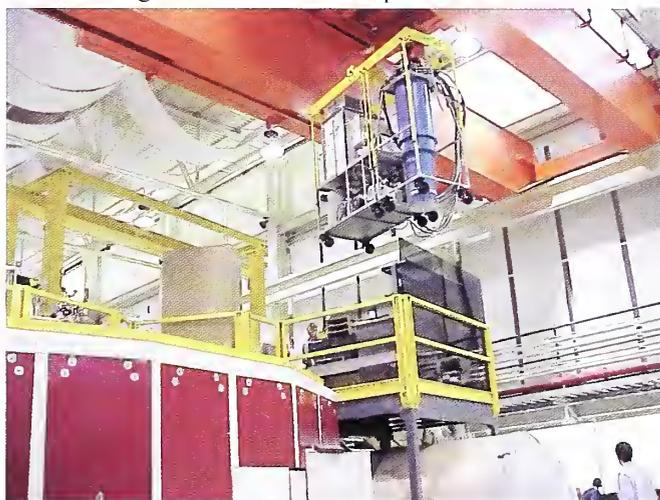
**Fig. 6.** Superconducting magnet/dilution refrigerator as it is being lifted onto the DCS spectrometer. The adjustable lifting frame compensates for the lifting point shifting in case liquid cryogenics are added.
