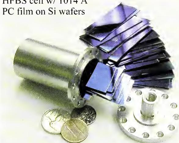
Fig. 1. A stack of 1014 Å PC films (notice the blue tint) on thin slabs of Si ready to go into the HFBS spectrometer.
