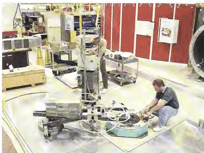
**Fig. 3.** Michael Murbach and Colin Wrenn conduct tests on the prototype floor system for a triple axis spectrometer.
