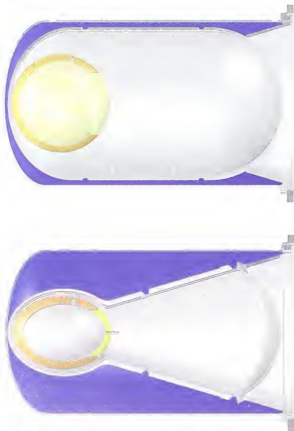
Fig. 1. Comparison between the original (top) and new designs for the liquid hydrogen cold source cryostat at NIST. Heavy water volume is indicated in blue, liquid hydrogen in orange, and hydrogen vapor in yellow.
