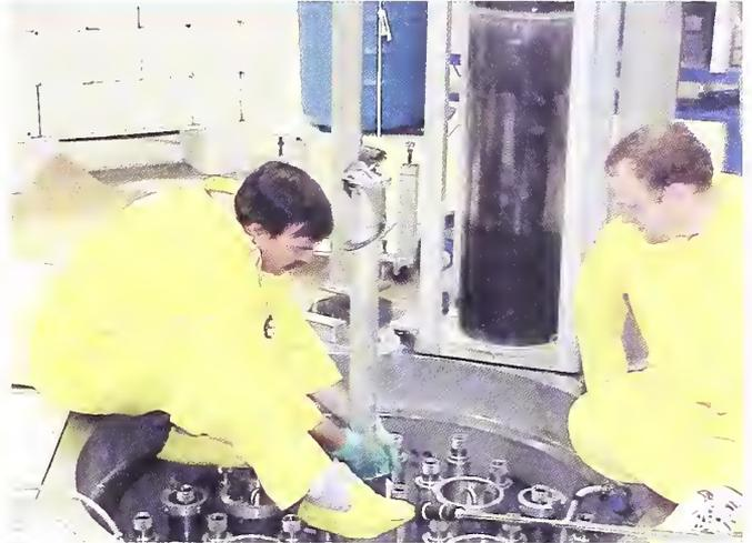
Fig. 1. Bill Mueller and Greg Heller of the reactor operations staff adjust the reactor power regulatory rod.
