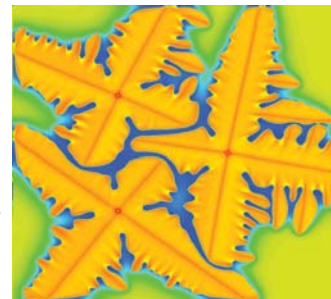
Figure 1. View of a phase field simulation of 4 alloy dendrites of differing orientation. The colors represent composition variations in the system, while orientation differences are evident from the axes of the dendrite trunks.
