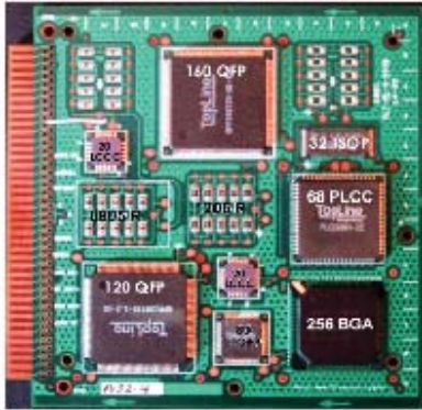
Figure 2. Reliability Test Vehicle used to test manufacturability and thermal fatigue resistance of a variety of surface mount components on printed circuit boards.
