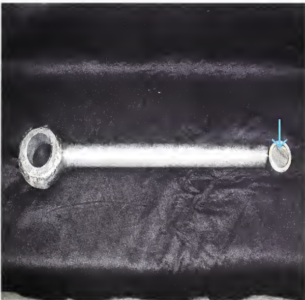
Figure 3. The failed pin and pin head showing fatigue fracture surface.
