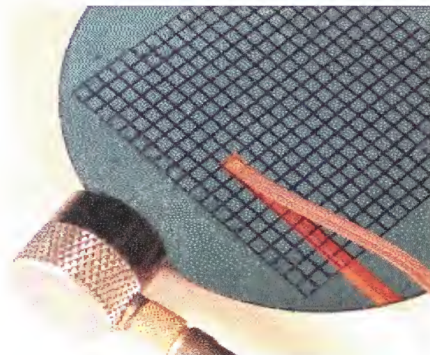
Figure 1. Photograph of the apparatus used to compare the theoretical model for a MUT with measurements on a combinatorial library formed by a Ni film on silicon.
