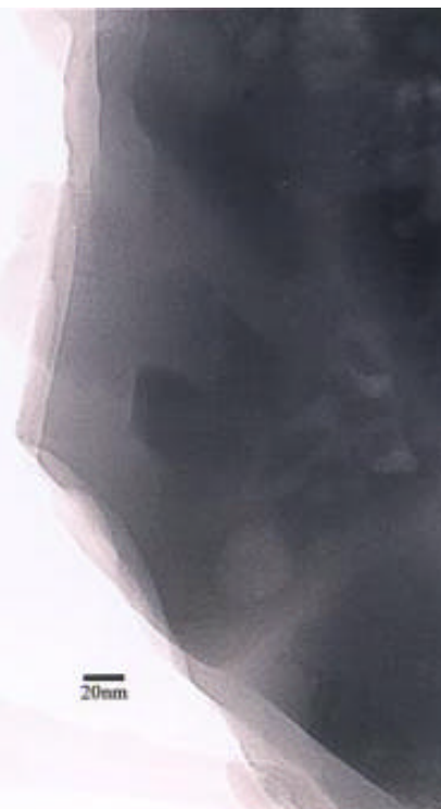
Figure 3 - Pure zeolite-NaX, without \text{Fe}_2\text{O}_3 clusters.
