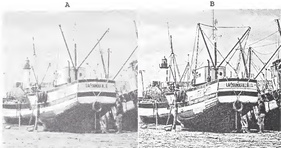
FIG. 11. Enhancement of boat image. APEX method with A = 4.0 on |\xi| \leq 250 , yields \alpha = 0.518155 , \beta = 0.215083 . Using these parameters with s = 0.01 , K = 1300 , and backwards continuation terminated at t = 0.5 , SECB method applied to image (A) produces image (B). Number 7 2 7 on side of boat in image (B) was not easily identifiable in image (A).
