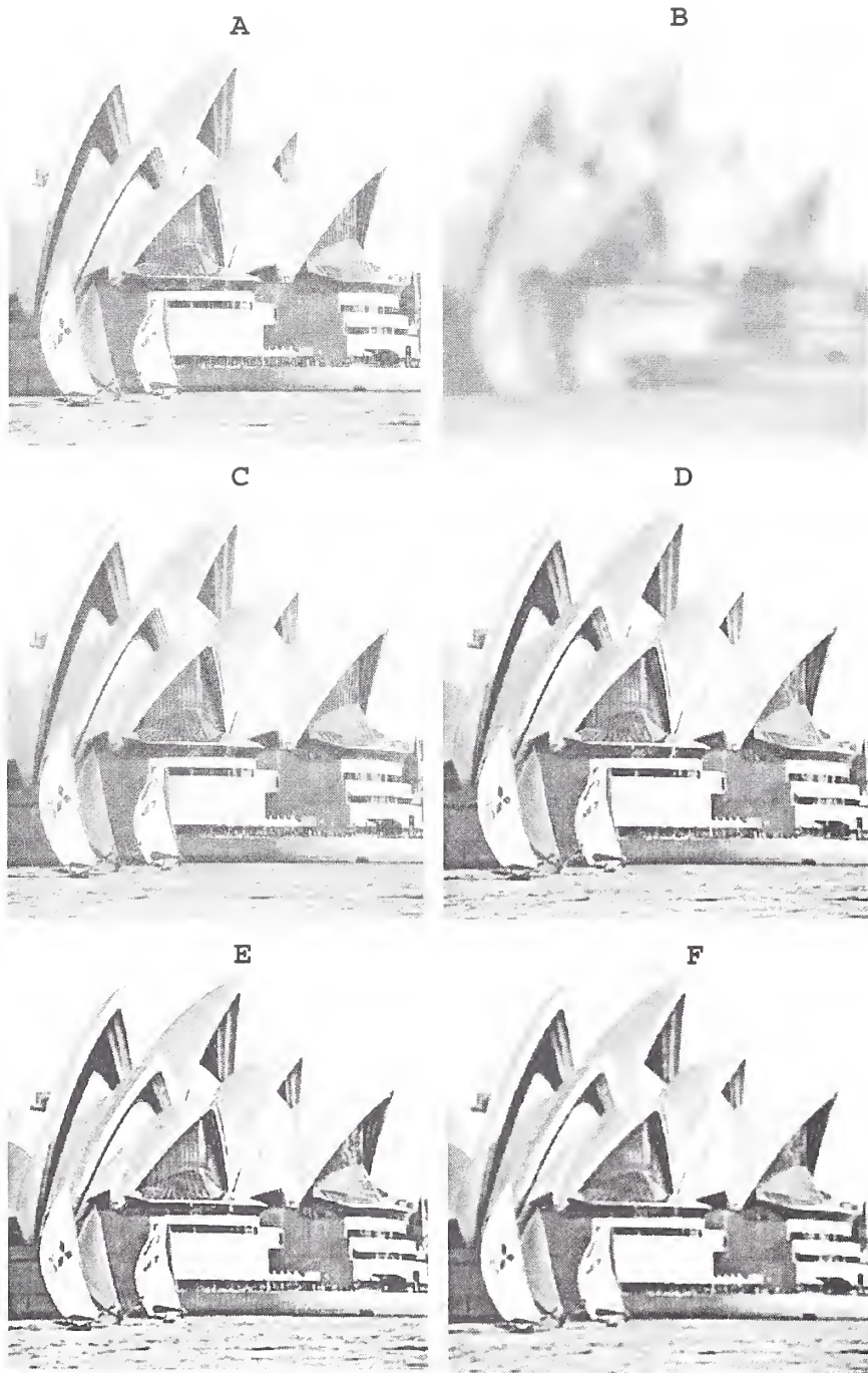
FIG. 1. Non uniqueness in blind deconvolution. Distinct point spread functions exist that produce high quality reconstructions from same blurred image. (A) Original sharp 512 \times 512 Sydney image. (B) Synthetically blurred Sydney image created by convolution with Lorentzian density with \alpha_0 = 0.075 , \beta_0 = 0.5 . Blurred image computed and stored in 64-bit precision. (C) Deblurring of image (B) using correct parameters \alpha = 0.075 , \beta = 0.5 . (D) Deblurring of image (B) using \alpha = 0.1301264 , \beta = 0.41298 . (E) Deblurring of image (B) using \alpha = 0.1950345 , \beta = 0.403889 . (F) Deblurring of image (B) using \alpha = 0.2360994 , \beta = 0.369666 . Notice that images (D), (E), and (F) were found using specific pairs (\alpha, \beta) where \alpha > \alpha_0 and \beta < \beta_0 . All deblurred images obtained using SECB procedure with s = 0.001 and K = 10000 .
