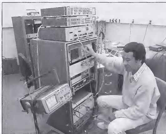
Yicheng Wang sets up an automated system for determining the frequency dependence of fused-silica capacitors.
