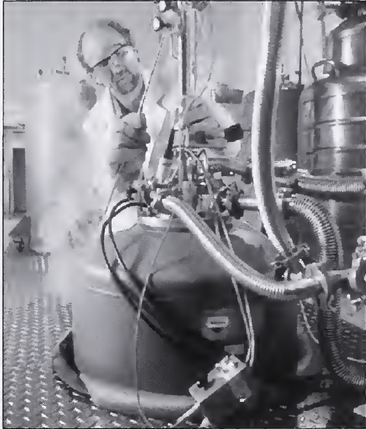
Physicist Rand Elmquist fills a cryogenic chamber with liquid helium in preparation for measuring the international standard for electrical resistance — the quantum Hall effect.
