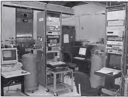
The NIST 10 V and 1 V Josephson voltage standard systems relocated in the new Advanced Measurement Laboratory.
