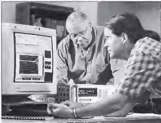
Robert Palm and Bryan Waltrip evaluate the performance of the NIST-developed Sampling Waveform Analyzer and its associated input probes for accurately measuring pulse waveforms.
