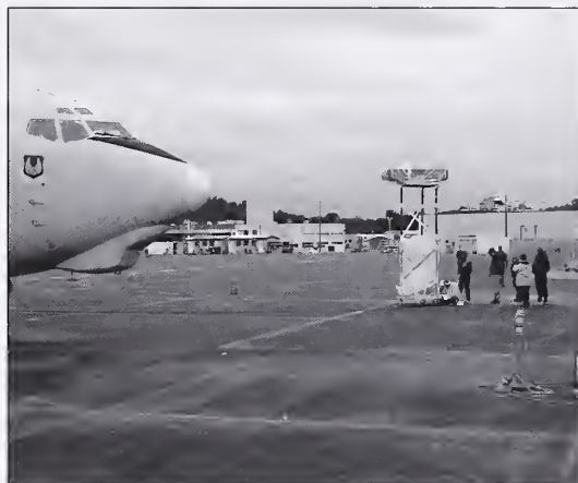
Evaluation of a U.S. Air Force early-warning aircraft using a portable NIST time-domain measurement system.
