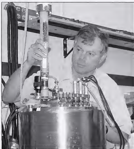
Loren Goodrich positioning probe with superconductor wire into the bore of a high-field superconducting magnet.
