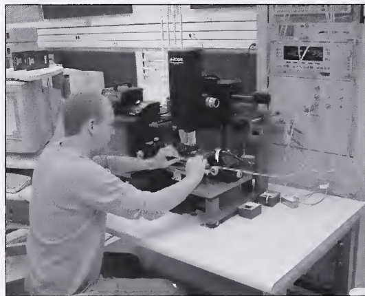
Jeffrey Jargon measures a commercial harmonic phase reference standard using the large-signal network analyzer.
