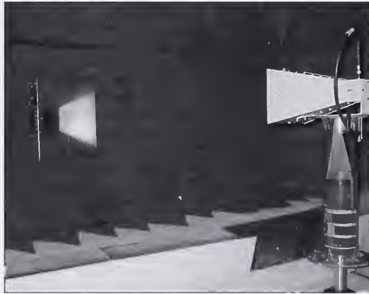
Antenna under test at NIST anechoic chamber facility.
