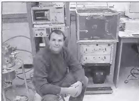
Mike Schneider next to cryogenic and room-temperature pulsed inductive microwave magnetometers.
