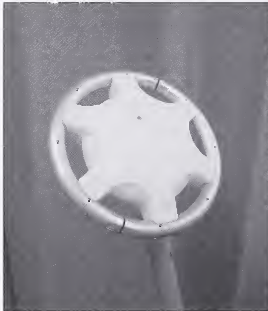
Double gap loop antenna system for simultaneous measurement of E and H.
