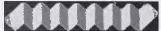
Micrograph of a zig-zag magnetoresistive element obtained by use of a scanning electron microscope with polarization analysis (SEMPA). With respect to the long axis of the sensor (the axis of current), light gray indicates magnetization at an angle of +45 degrees, dark gray at an angle of -45 degrees. The magnetic domain patterns were also accurately modeled with NIST's Object Oriented MicroMagnetic Framework (OOMMF).
