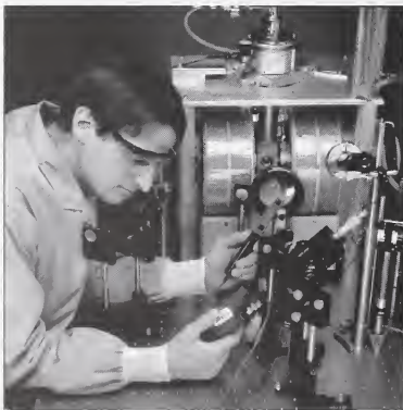
Electronics engineer Tony Kos aligning optics for pump/probe measurements of spin populations in GaAs. Photo © 2002 Geoffrey Wheeler.
