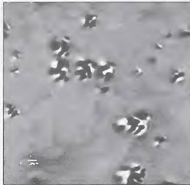
MFM image of Co particles in a SiCN matrix. The alternating white and black regions show the magnetic domain structure of the Co particles. This nanostructured magnetic material has very high thermal and mechanical stability.
