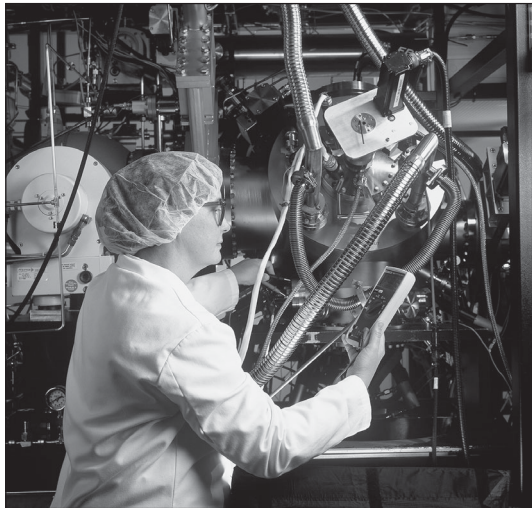
Gas-source molecular beam epitaxy growth system used to study III-V crystal growth by Kris Bertness (in picture) and others at NIST. © Geoffrey Wheeler
