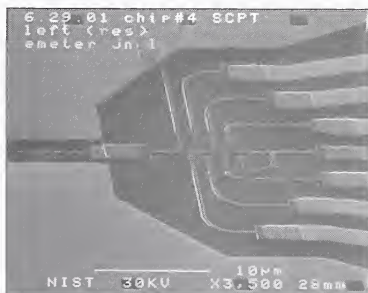
SEM micrograph of our first 7-junction SCPT pump. The junctions, which are less than 50 nm on a side, are too small to be seen in this picture but are located on the central line near each gate electrode.
