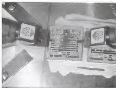
View of two 40 GHz probes and a sample of YBCO devices in the probe station. Devices such as these are used for the nonlinear phase measurements and the microwave power limiter.
