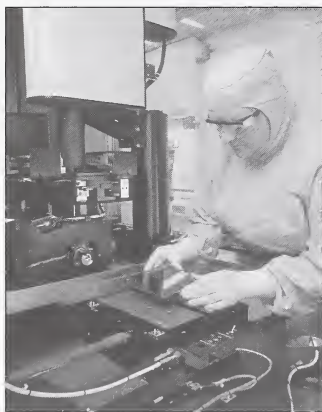
Maggie Crews inspects a mask generated in our new Optical Pattern Generator.
