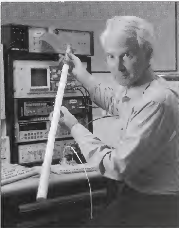
Clark Hamilton showing the probe for the 10 V conventional Josephson voltage standard system developed at NIST and used throughout the world for calibration of Zener voltage references.
