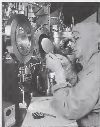
Leila Vale examines a 76 mm Nb/Al 2 O 3 /Nb trilayer wafer that will be used for Josephson junction circuit fabrication.
