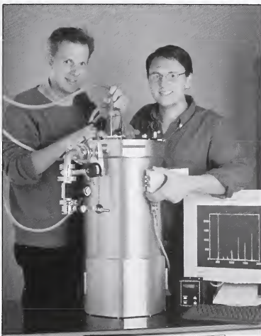
Gene Hilton and Steve Deiker standing by an Adiabatic Demagnetization Refrigerator (ADR). The ADR is used to cool our transition edge sensor (TES) x-ray detector down to about 1/10^{10} of a degree above absolute zero. The TES is used to provide extremely sensitive x-ray microanalysis of materials.
