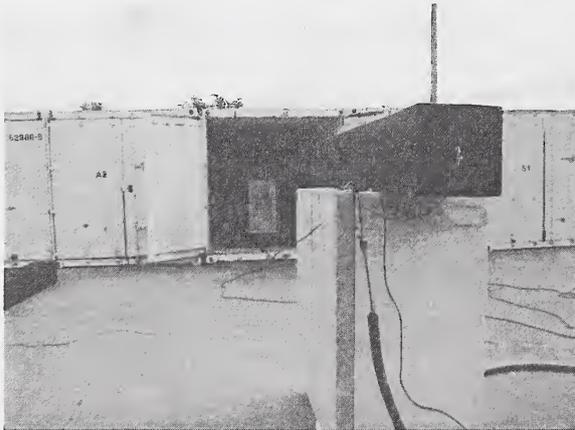
Figure 19. Antenna measurements in iso-container to simulate actual aircraft conditions.
