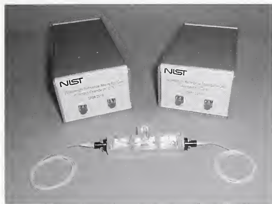
Wavelength calibration Standard Reference Materials.
