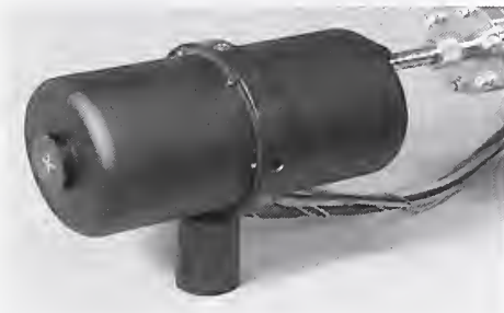
The C-Series Calorimeter, originally developed in the 1970s for use with cw lasers in the range from 50 \mu\text{W} to 1 W and 0.4 \mu\text{m} to 2 \mu\text{m} wavelength. Improved versions in current use for calibrations.
