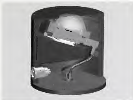
A three-dimensional representation of a new pyroelectric-based radiometer head for infrared optical measurements as part of a collaboration with the NIST Optical Technology Division. The critical detector element and gold-black coating are being developed in the Optoelectronics Division.
