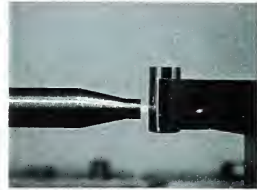
Ferrule diameter measurement with laser micrometer.
