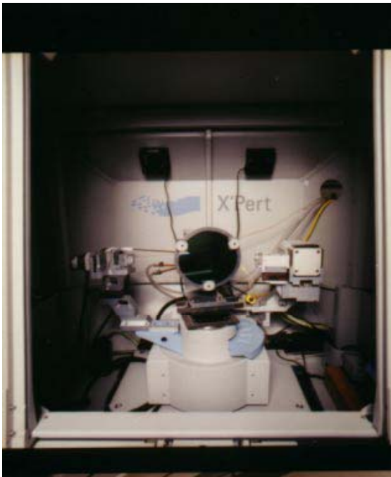
Photograph of the interior of the NIST high-resolution x-ray reflectometer with a silicon wafer with a low-k dielectric thin film.
