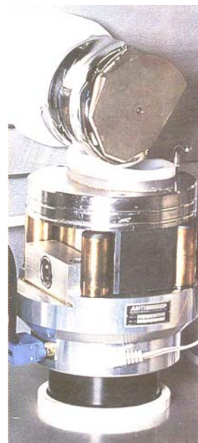
The NIST Orthopedics Research Consortium, whose member companies manufacture 80% of orthopedic total joint replacement products sold in the U.S., developed a new wear testing apparatus for accelerated screening of new materials without compromising the basic wear mechanisms that take place in the human body.
