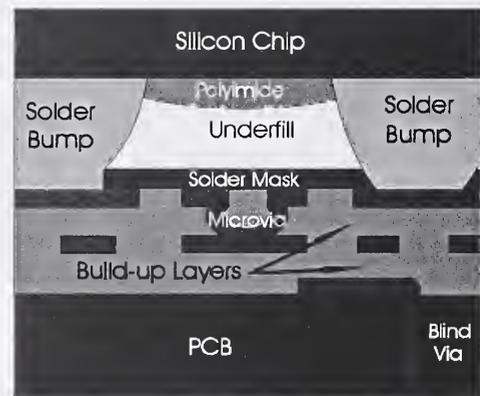
Figure 1. Structure of a flip chip package showing the solder bump connections and the multilayer wiring structure.
