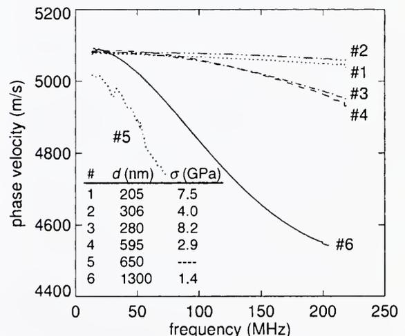
SAW dispersion relations for Si samples with TiN films. The thickness  $d$  and residual stress  $\sigma$  for each film are shown.
