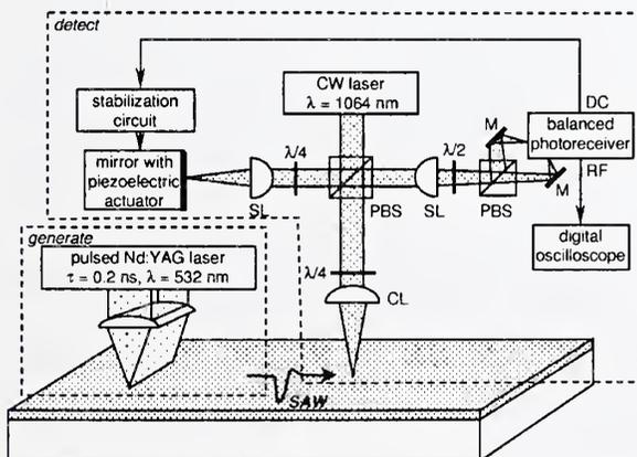
Schematic of laser-ultrasonic SAW apparatus.
