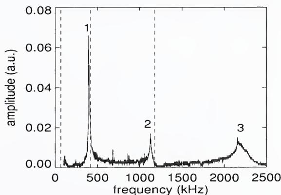
First three flexural resonances for a rectangular Si cantilever in contact with  $\langle 100 \rangle$  Si. Dashed lines indicate the first three free-space resonances.
