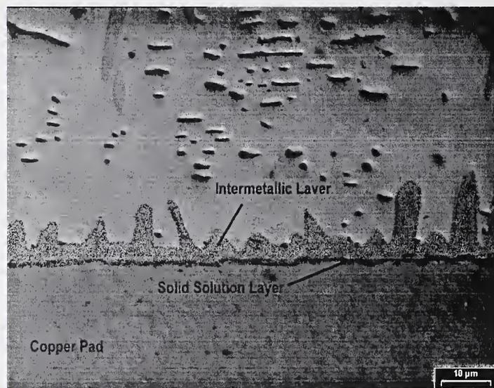
*Figure 1. Optical micrograph of the copper-solder interface. Adjacent to the copper (at the bottom) is a 1  $\mu\text{m}$  thin darker region, most likely Cu-rich-Sn solid solution, followed by the irregularly shaped Cu-Sn intermetallic layer, which ranges between 5 and 10  $\mu\text{m}$  thick.*
