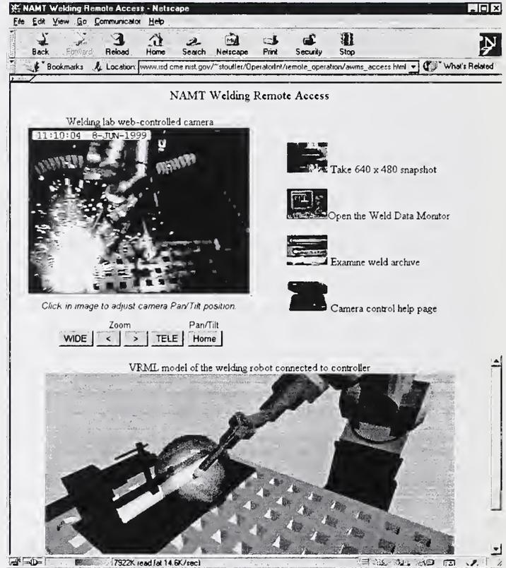
**Figure 1: The video image of the part as it is being welded and a solid model image of the robot are displayed on a web page.**
