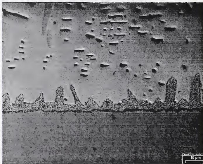
*Figure 1. Optical micrograph of the copper-solder interface. Adjacent to the copper (at the bottom) is a 1  $\mu m$  thin darker region, most likely Cu-rich-Sn solid solution, followed by the irregularly shaped Cu-Sn intermetallic layer, which ranges between 5 and 10  $\mu m$  thick.*
