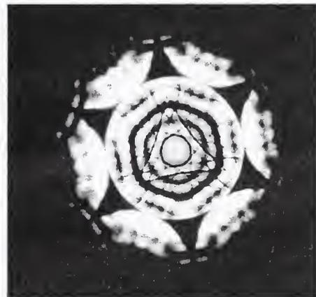
Figure 1. Convergent-beam electron diffraction pattern from copper, showing (111) crystal orientation and high-order diffraction lines used for measuring lattice parameters.
