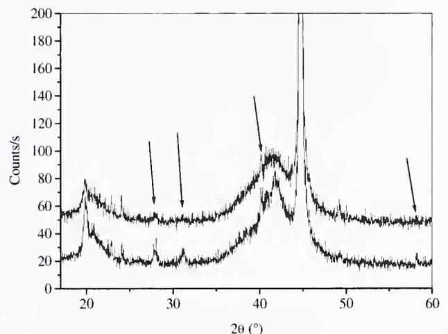
Figure 1. Diffraction patterns of optimally annealed (lower) and overheated (upper) samples. Arrows mark positions of affected diffraction lines.
