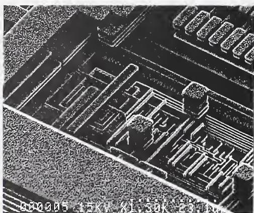
Figure 1. IBM CMOS 75 damascene copper interconnect structure.
