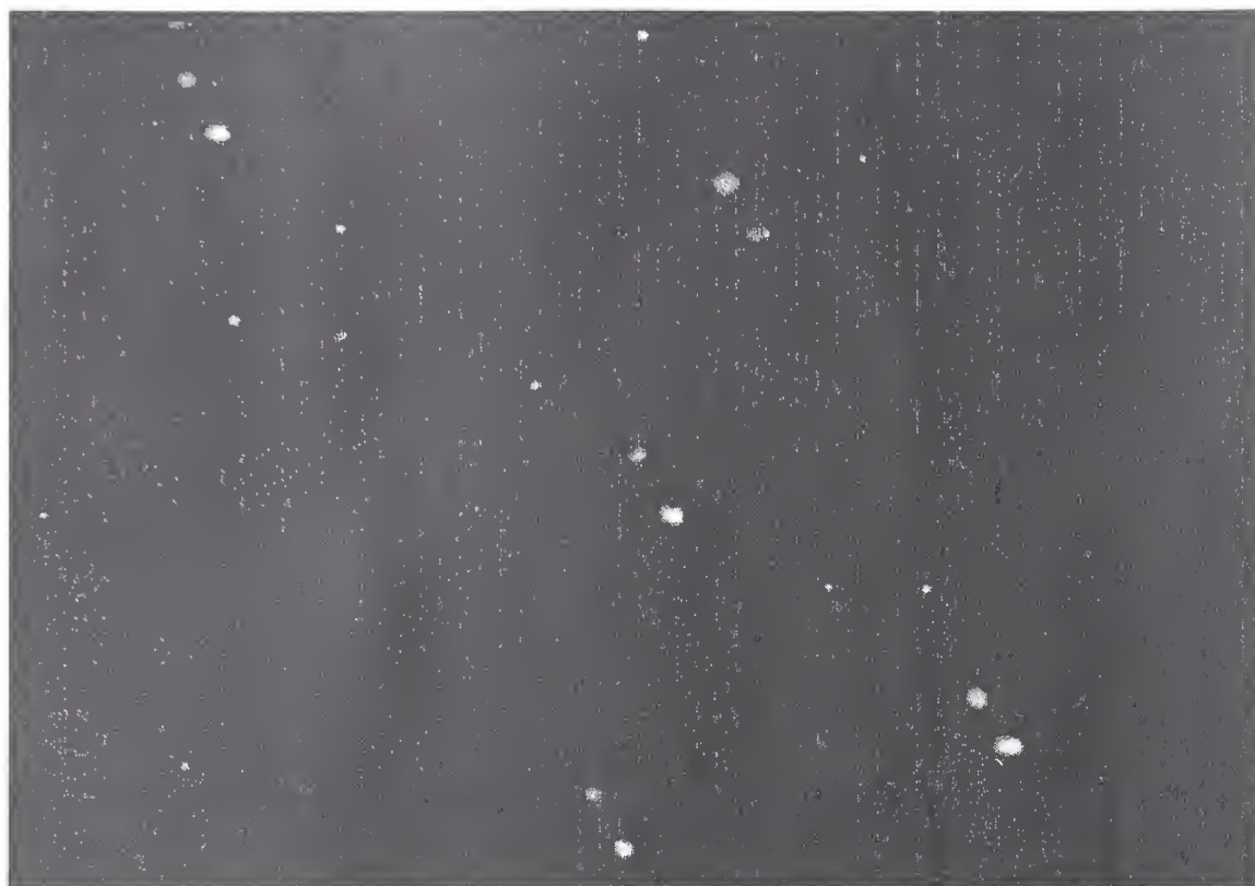
Fig. 6: Low Laser Power at 532nm (10 mJ/shot). High Laser Power at 355nm (120 mJ/shot). Imaged area: 84mmX118mm.
