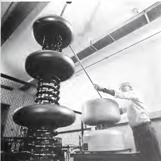
Martin Misakian connects a high voltage dc divider to a high voltage power supply.
