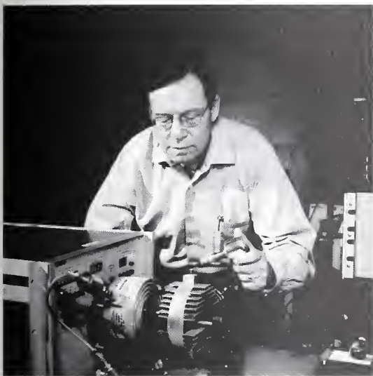
Joe Kinard running new NIST Special Tests for the ac-dc difference of 100 A ac current shunts.
