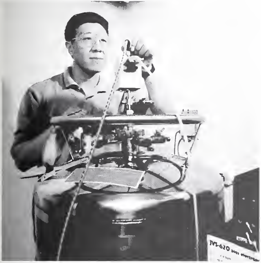
Yi-hua Tang installs the cryoprobe in the 1 Volt programmable Josephson array voltage standard.
