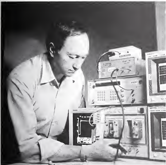
Don Larson measuring the step response on a fast pulse generator under the NIST Special Test service for fast repetitive pulse transition parameters.
