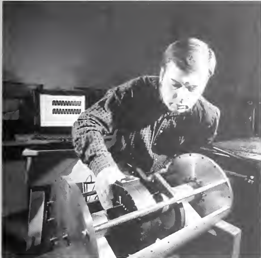
Eric Simmon installing an optical current sensor in a high-current coaxial cage.
