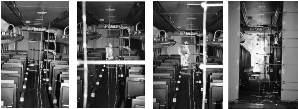
Figure 10. Amfleet I Test Car - Typical Medium T-squared Gas Burner Fire Growth
