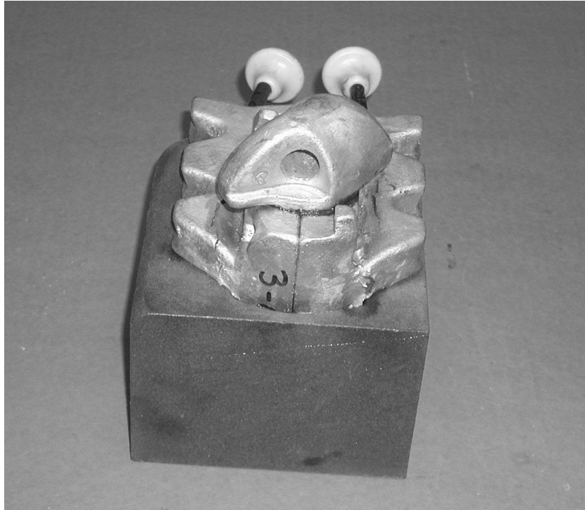
Figure 5.9 Specimen CON-T-N after Compression Test (Note: twistlock depressed into corner fitting.)
