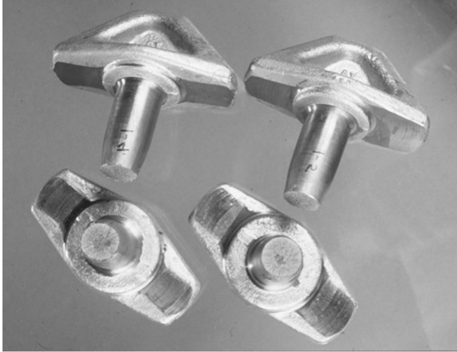
Figure 5.20 Brittle Failure of Tensile Test Specimen (ASM-T-N)
