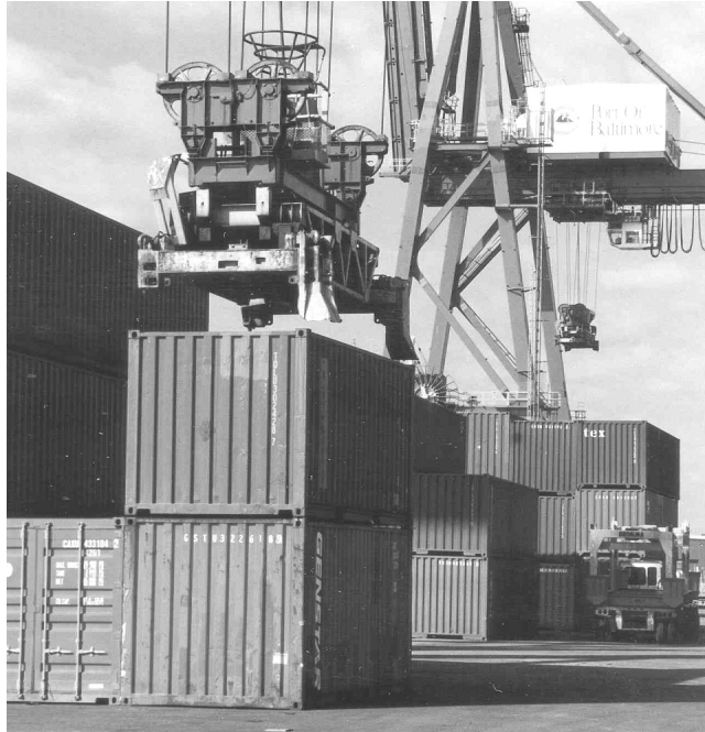
Figure 2.1 Lifting of Containers by Gantry Crane
