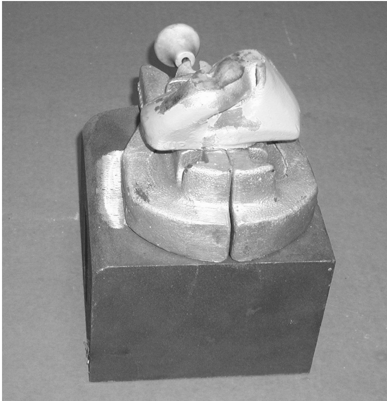
Figure 5.10 Specimen P&H-T-N after Compression Test (Note: cracks in intermediate plate)
