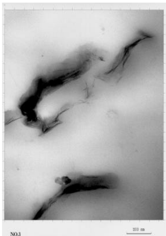
Figure 20. TEM of PP/5 % MMT (SCPX 1980) showing intercalated tactoid structure.
