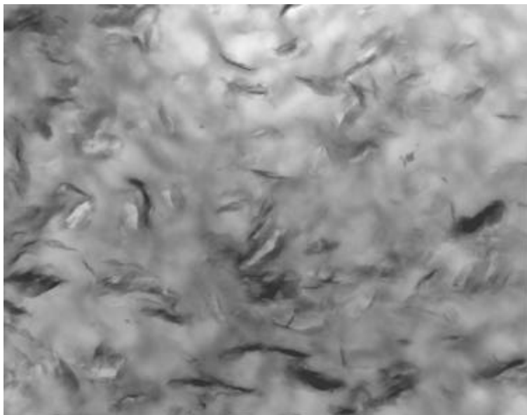
Figure 3. TEM of PA-6/5 % MMT (SCPX 2171) showing the intercalated tactoids dispersed in the PA-6.
