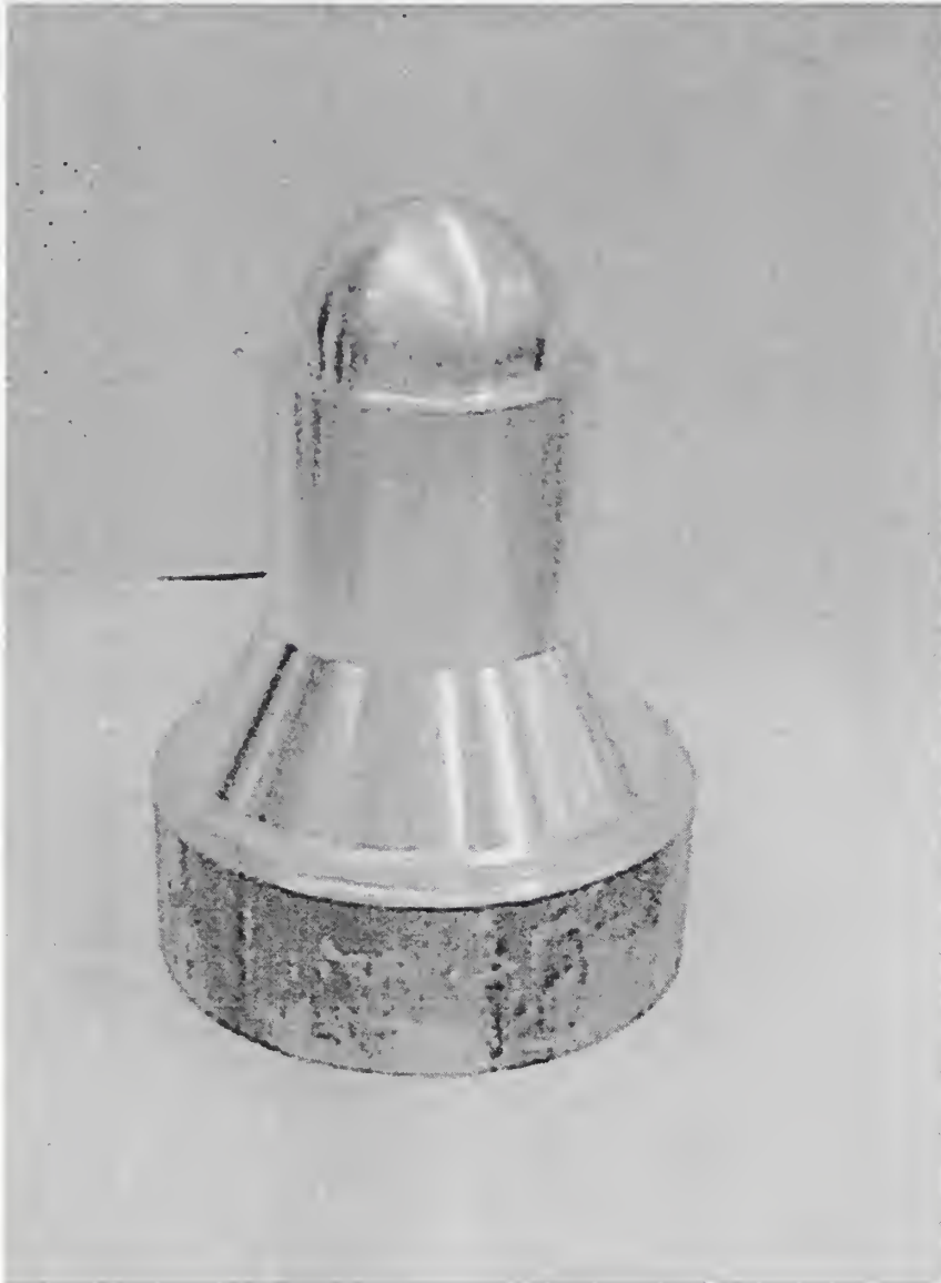
Figure 3: Part with Hemispherical Dome used to Test Algorithm
