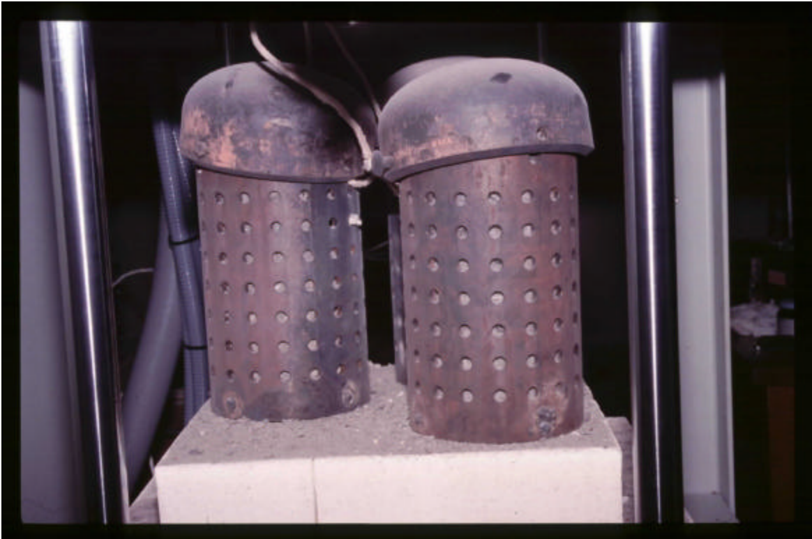
Figure 22 Explosion resistant steel shells in high temperature furnace.
