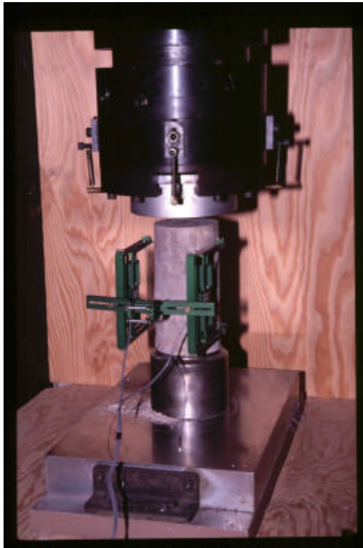
Figure 3 Compressive strength apparatus.
