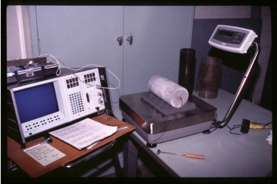
Figure 2 Apparatus for measuring resonant frequency.
