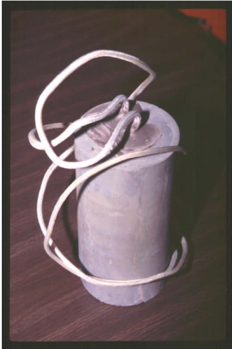
Figure 7 Example of concrete specimen used in heating characteristics study.
