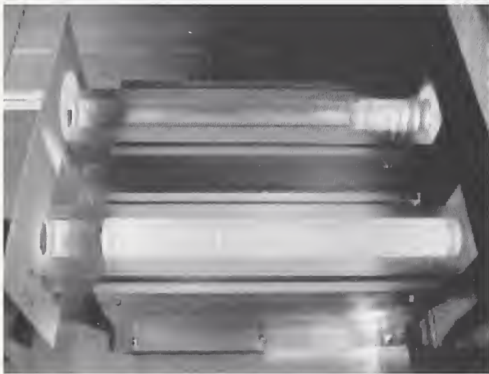
FIGURE 1. Now installed in the pre-sample flight path of the NG-7 30-meter SANS instrument are two sets of \text{MgF}_2 biconcave lenses that can be inserted into the beam under computer control. The 28-lens array in the foreground focuses 8.44 \text{ \AA} neutrons at a distance of 15 m from the lenses, and the 6-lens set focuses 18 \text{ \AA} neutrons at the same distance. Each lens is 25 mm in diameter, has a radius of curvature of 25 mm, and is 1 mm thick in the center.
