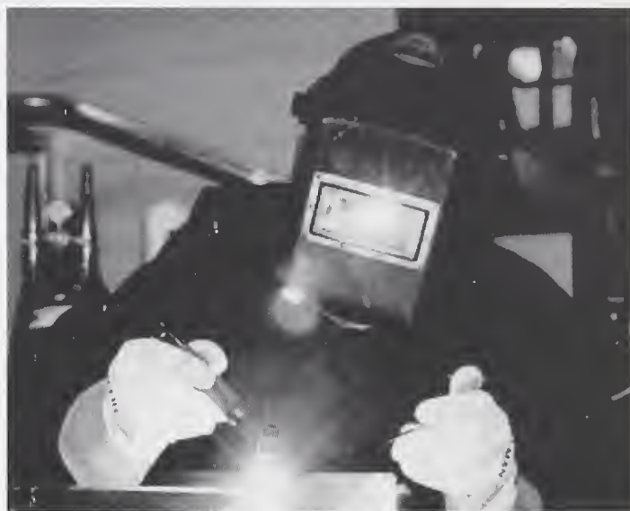
FIGURE 6. NCNR Mechanical Engineering Technician, Scott Slifer, welds the aluminum moderator vessel for the advanced hydrogen cold source.
