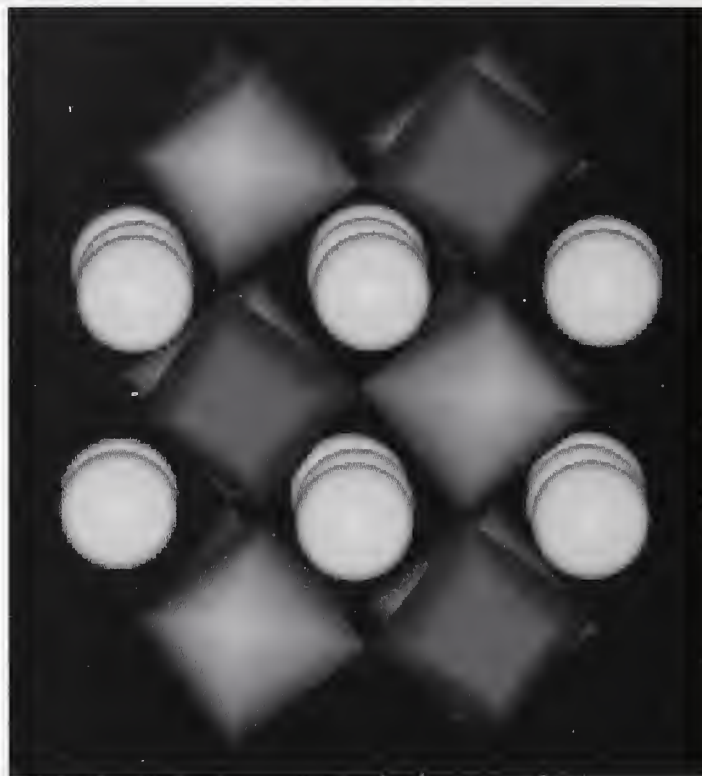
FIGURE 1. The low temperature structure of \text{CaFeO}_3 . The green spheres depict the calcium ions. The other shaded objects represent iron centered octahedra, where an oxygen atom can be found at each vertex and an iron atom at the center of each octahedron. The purple and blue objects represent \text{Fe}^{3+} centered and \text{Fe}^{5+} centered octahedra respectively.
