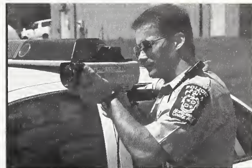
Law enforcement officer using a traditional down-the-road radar gun during speed enforcement operations.
