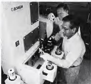
Performing in-situ X-ray emission measurements.
