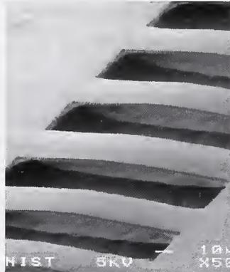
**Fixed-fixed beam test structure array for measurement of mechanical strain and interconnects in multilayer structures.**
