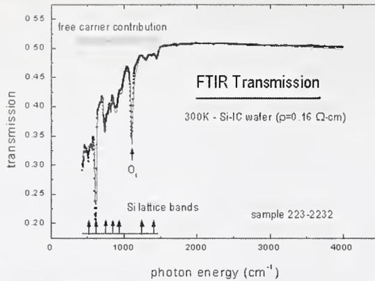
**Infrared transmission spectrum from a conducting Czochralski wafer: data (line) and model calculations (dots) are shown. Note that all the observed features Si lattice, oxygen impurity and the charge carriers are observed and reproduced by the model.**
