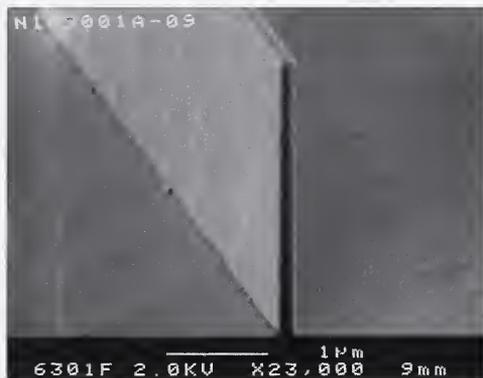
Part of an electrical test structure formed in single-crystal silicon. This structure, developed in cooperation with Sandia National Labs, will help to resolve differences between electrical, SEM, and optical CD measurements.
