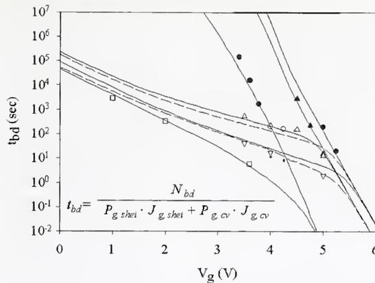
Plot above shows model and data for the combined effects of substrate hot-electron injection and high voltage stress on the lifetime of ultra-thin gate oxides.
