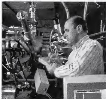
Performing *in-situ* X-ray emission measurements.
