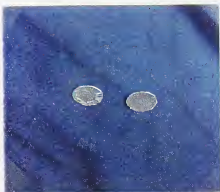
CV5-10 source disks [pair of U235 metal source disks wrapped in aluminum foil]
