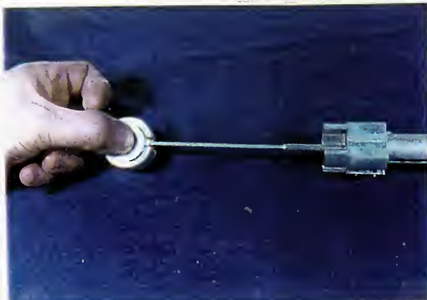
CIb Push rod [procedure for using tool SITa to remove press-fit capsule holder cap]
