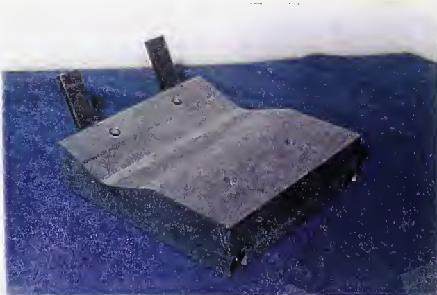
SCRc: Cylinder cradle with rollers
