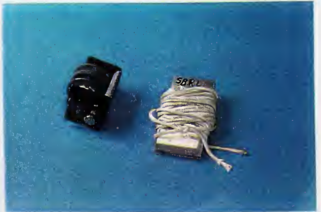
SBRi: Pulley assembly and pull cord
