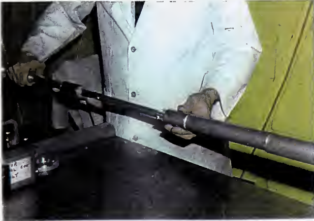
CI Detector capsule insertion assembly [inserting CI into source insertion assembly SI]
