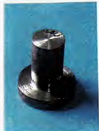
SB1j: Steel shield plug for reduction tube, SB1b
