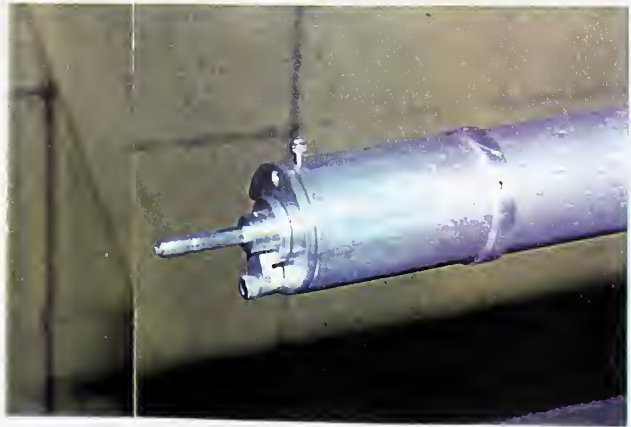
CIb Push rod [CI inserted into SI, endview showing end stop, clamp, and attachment screw]
