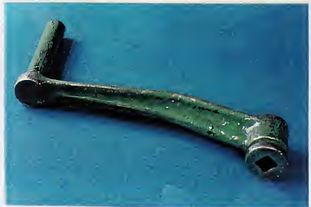
LTa: Wrench for lift sprocket
