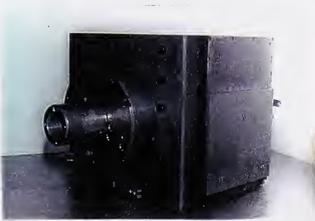
SB1/SB1a/SB1b/SB1g: Inner lead shield box complete with 8" dia. cyl. (SB1a), penetration reduction tube w/attachmnt screw (SB1b), eyebolt for pull cord, cinch pin (SB1g)
