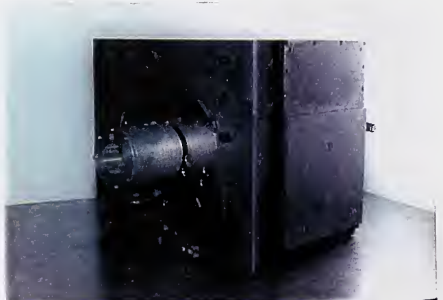
SB1: Inner lead shield box w/ CFS guide tube (SB1d) in place
