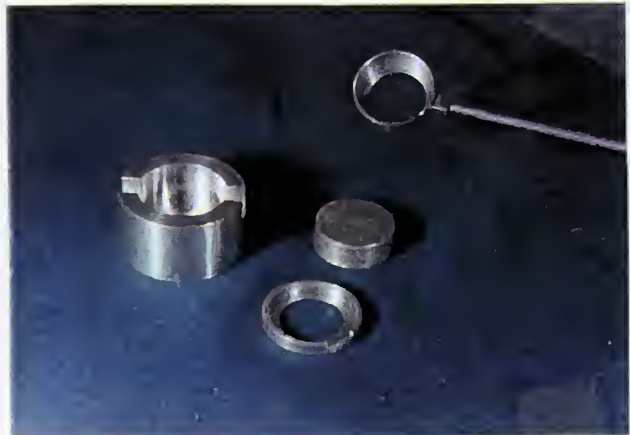
CIb Detector capsule holder assembly [capsule holder, detector capsule (CC), holder cap; left: cap removal tool (SITa)]
