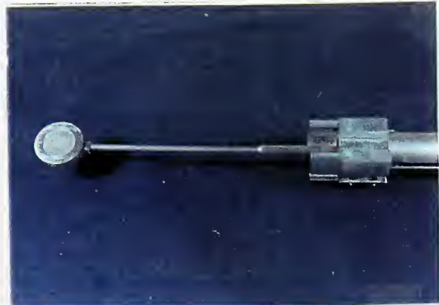
CIb Push rod [extended w/ detector capsule holder & cap]
