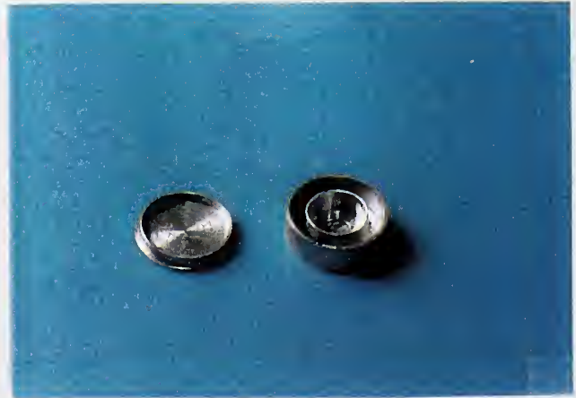
CC Cadmium capsule with "hat" for detector foil assembly
