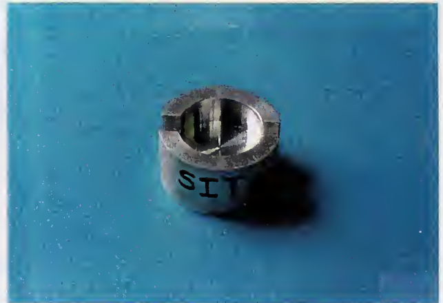
SITa Removal tool for capsule-holder cap
