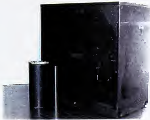
SB3: Middle shield box w/ lead closure plug, SB3a, and steel plug, SB3b
