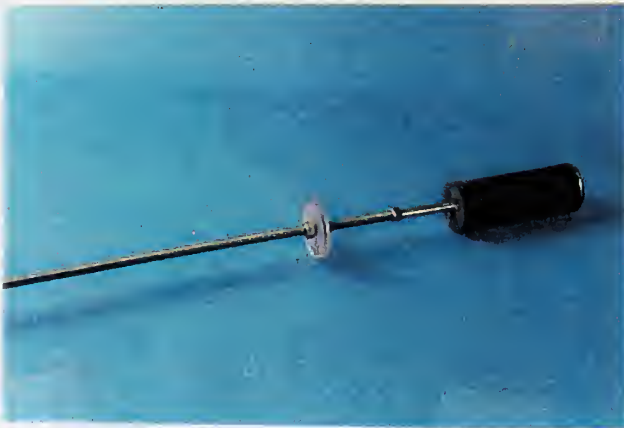
SB1i: Lead shield plug (2.7" dia.) for SB1a
