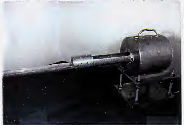
PSa: Portable lead shield w/ extension piece, PSB: Dolly for portable shield
