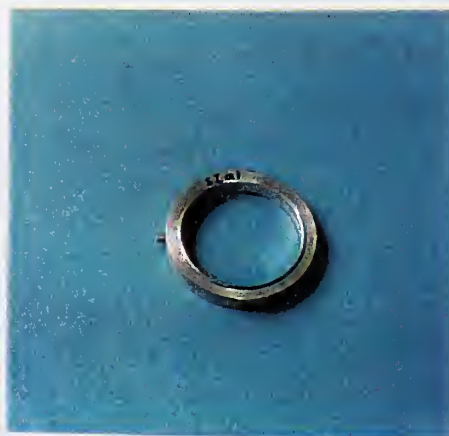
SIa1 stop ring for source insertion tube
