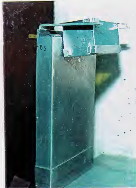
BS: Body shield attached to lift table w/glass brick in place for viewing
