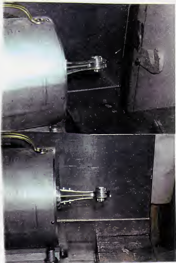
SIb1,2 source mounting tabs [upper and lower source tabs protruding from portable shield with detector capsule inserted]
