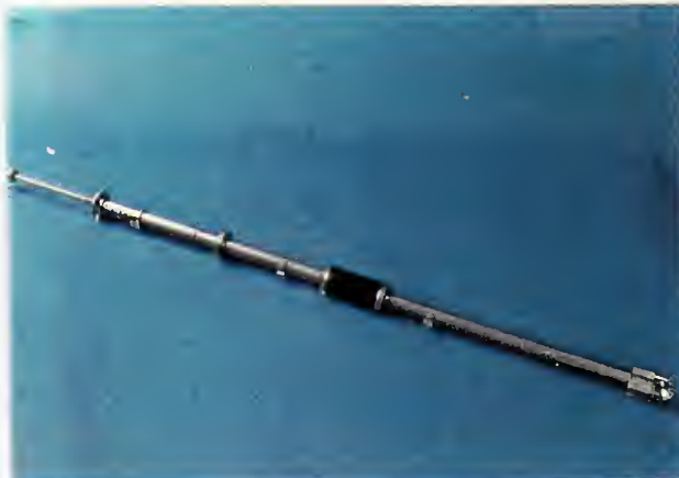
CIa Insertion guide for detector capsule push rod [capsule insertion assembly with push rod withdrawn]
