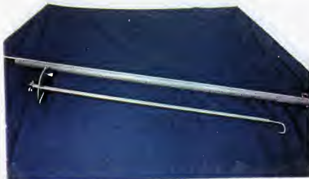
GRe: Rod and wishbone attachment for removing cylinder GC1,2
