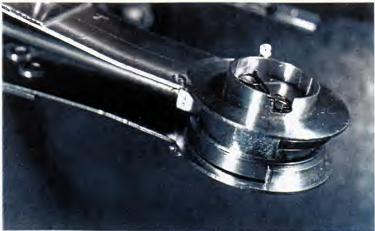
Fig. B1-4. Close-up of the source tabs with detector capsule inserted. The wrapped fission source disk is under the coiled wire spring. [More recently, the fission disks are held in place with an aluminum twist lock.]
