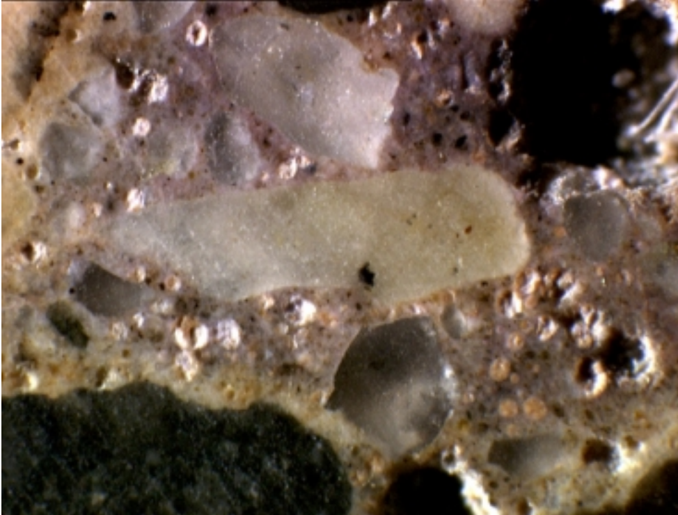
Figure 11. Iowa 175 Core 2 base mortar microstructure exhibiting partial filling of the entrained air void system. Micrograph field width: 4 mm
