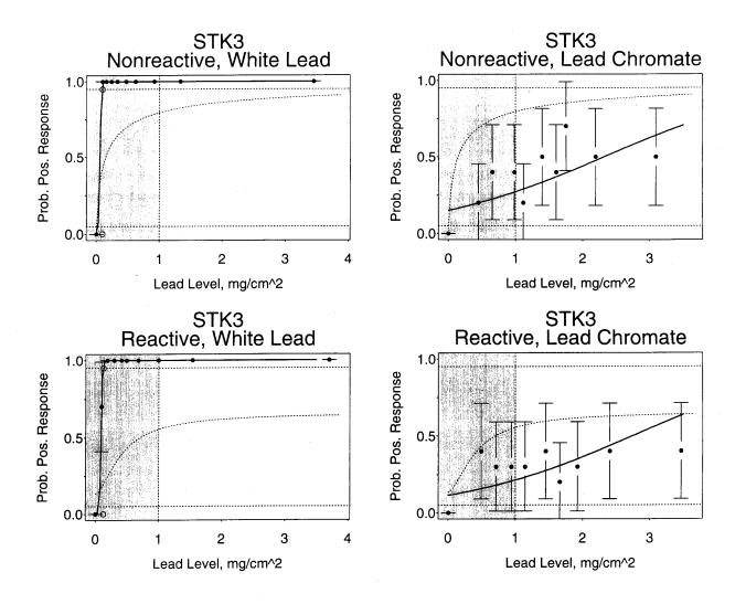
Figure 10. Comparison of the Results of the NIST Laboratory Data With Those of the EPA/HUD Field Data [8] for Spot Test Kit 3. (The solid and dashed curves represent the NIST and EPA/HUD data, respectively.)
