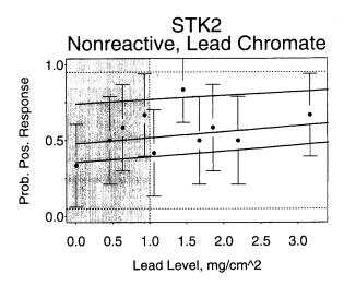
Figure 2. Probability of a Positive Response Versus Lead Level for Spot Test Kit 2 (STK2) for Each Operator. (The filled circles represent the proportions of positive responses at a given lead level, and the error bars are the associated 95 % binomial confidence intervals. The two horizontal dashed lines represent the 0.5 and 0.95 probabilities of a positive response. Circles are the 0.95 probability point for each operator; they are repeated above the horizontal axis for clarity.)
