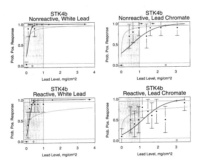
Figure 11. Comparison of the Results of the NIST Laboratory Data With Those of the EPA/HUD Field Data [8] for Spot Test Kit 4. The Comparison was Made for the STK4b Procedure. (The solid and dashed curves represent the NIST and EPA/HUD data, respectively.)
