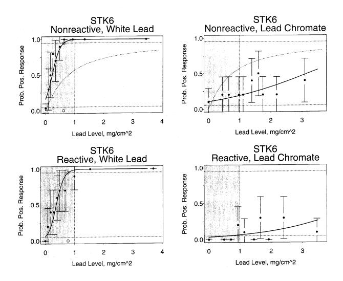
Figure 12. Comparison of the Results of the NIST Laboratory Data With Those of the EPA/HUD Field Data [8] for Spot Test Kit 6. The EPA/HUD Study did not Include Data for a Reactive Substrate. (The solid and dashed curves represent the NIST and EPA/HUD data, respectively.)
