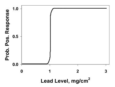
Figure 9. Example of the Ideal Performance of a Spot Test Kit for Determining Lead-Based Paint.
