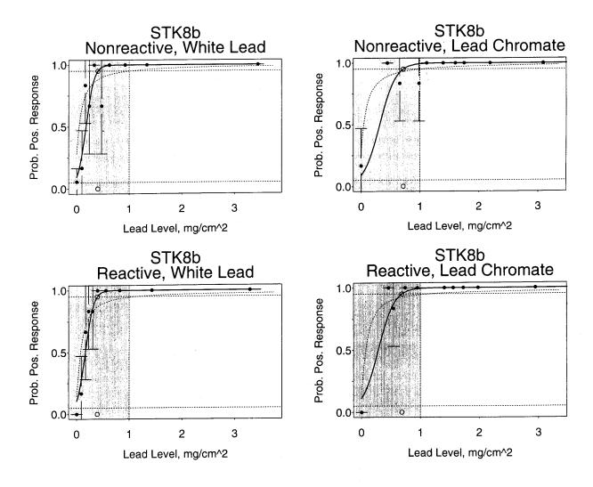
Figure 14. Comparison of the Results of the NIST Laboratory Data With Those of the EPA/HUD Field Data [8] for Spot Test Kit 8. The Comparison was Made for the STK8b Procedure. (The solid and dashed curves represent the NIST and EPA/HUD data, respectively.)
