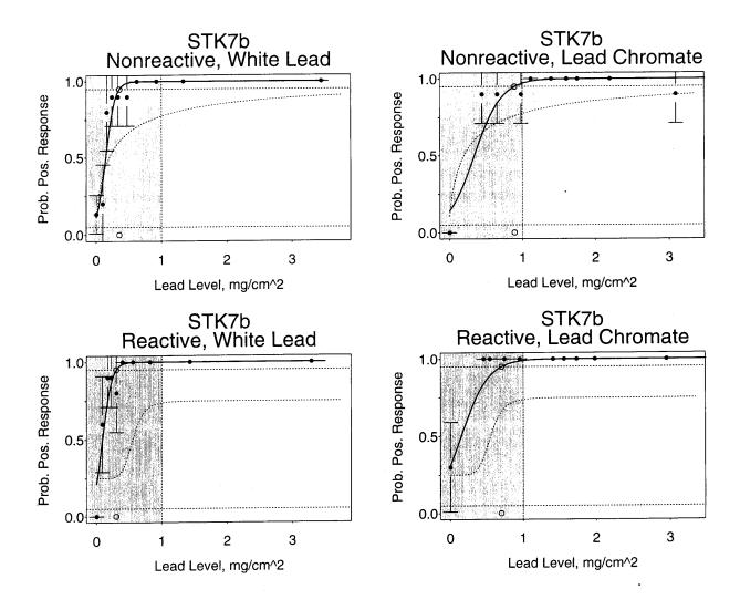
Figure 13. Comparison of the Results of the NIST Laboratory Data With Those of the EPA/HUD Field Data [8] for Spot Test Kit 7. The Comparison was Made for the STK7b Procedure. (The solid and dashed curves represent the NIST and EPA/HUD data, respectively.)
