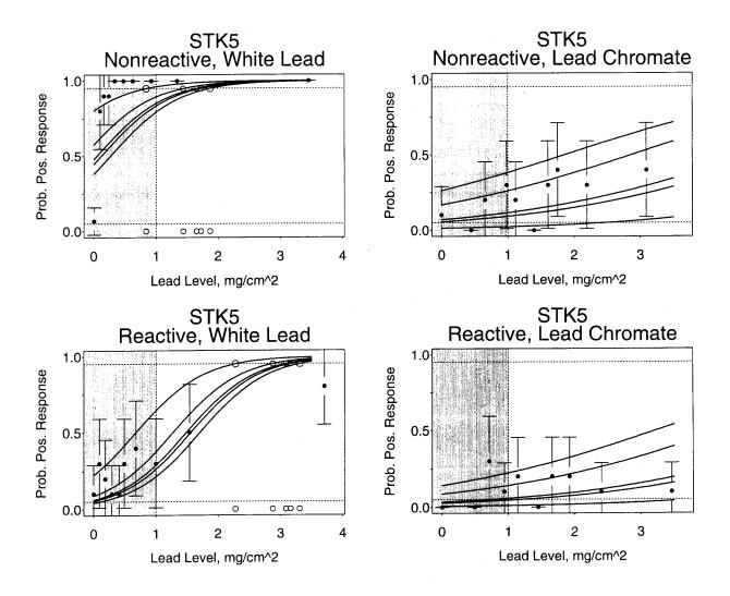
Figure 5. Probability of a Positive Response Versus Lead Level for Spot Test Kit 5 (STK5) for Each Operator. (The filled circles represent the proportions of positive responses at a given lead level, and the error bars are the associated 95 % binomial confidence intervals. The two horizontal dashed lines represent the 0.5 and 0.95 probabilities of a positive response. Circles are the 0.95 probability point for each operator; they are repeated above the horizontal axis for clarity.)
