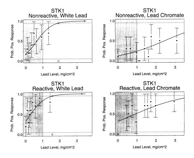
Figure 1. Probability of a Positive Response Versus Lead Level for Spot Test Kit 1 (STK1) for Each Operator. (The filled circles represent the proportions of positive responses at a given lead level, and the error bars are the associated 95 % binomial confidence intervals. The two horizontal dashed lines represent the 0.5 and 0.95 probabilities of a positive response. Circles are the 0.95 probability point for each operator; they are repeated above the horizontal axis for clarity.)
