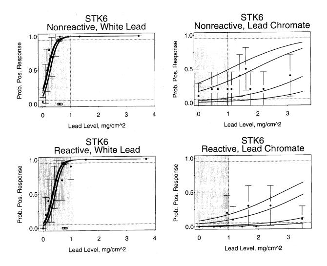
Figure 6. Probability of a Positive Response Versus Lead Level for Spot Test Kit 6 (STK6) for Each Operator. (The filled circles represent the proportions of positive responses at a given lead level, and the error bars are the associated 95 % binomial confidence intervals. The two horizontal dashed lines represent the 0.5 and 0.95 probabilities of a positive response. Circles are the 0.95 probability point for each operator; they are repeated above the horizontal axis for clarity.)
