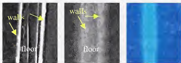
Fluorescence images showing localization of channel charge (bright spots on images). Channels approximately 50 \mu\text{m} wide. (A) room temperature imprinted; (B) hot imprinted; (C) laser ablated channel.
