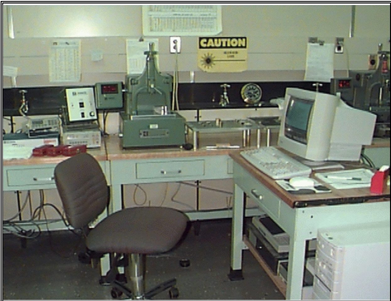
Figure 2.1-1 Gage Block Calibration and Measurement Workstation
