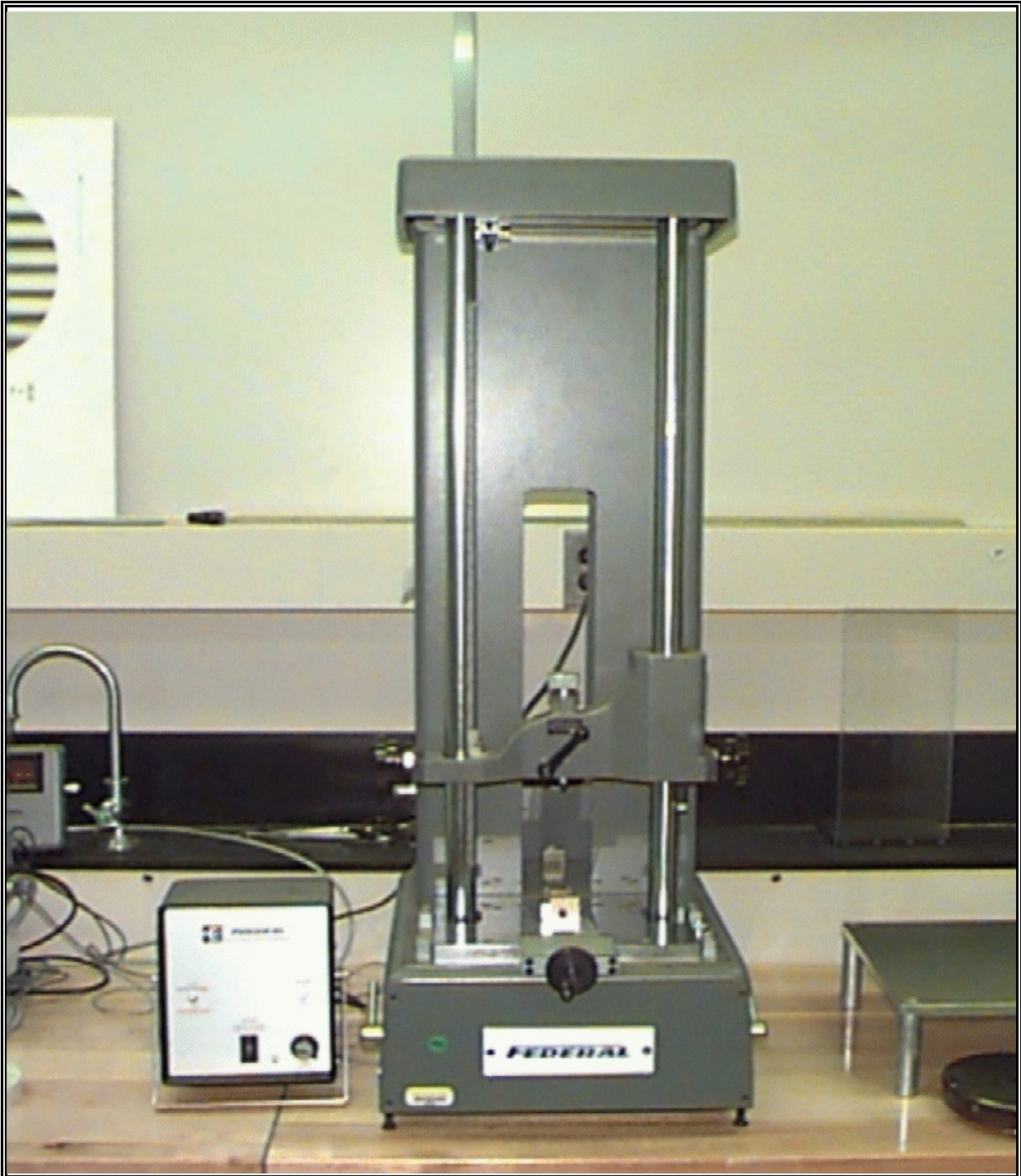
Figure 2.3-2 Long Gage Block Comparator
