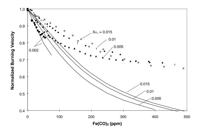
Figure 9: Calculated and measured normalized burning velocities for flames inhibited by Fe(CO)<sub>5</sub> for various H<sub>2</sub> concentrations.  $\phi$ =1.0 and  $X_{O_2ox}$  = 0.24.
