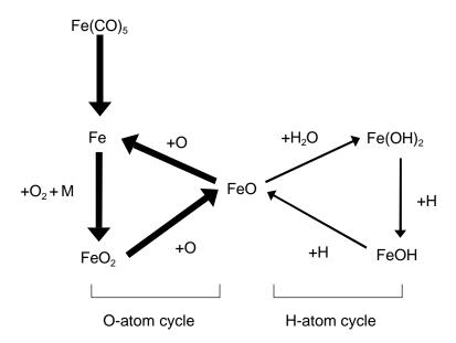
Figure 4: Schematic diagram of reaction pathways in CO-H<sub>2</sub>-O<sub>2</sub>-N<sub>2</sub> flames based on the gas-phase mechanism of Ref. [8]. Thicker arrows correspond to higher reaction flux. Reaction partners are listed next to each arrow.
