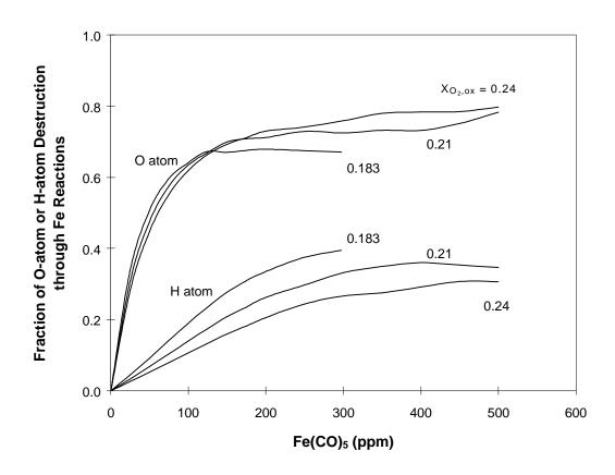
Figure 6: Calculated fractional H-atom and O-atom flux through key iron reactions at  $X_{H_2} = 0.01$  and varying  $O_2$  concentrations.
