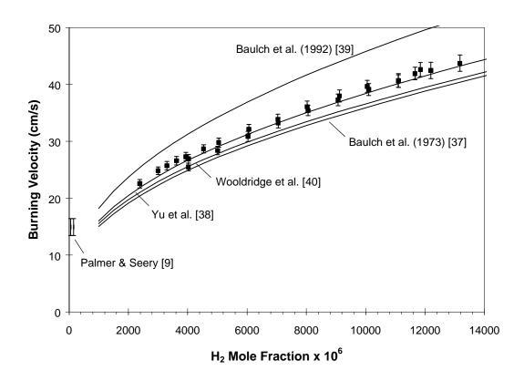
Figure 1: Comparison of measured and calculated burning velocities of stoichiometric CO- $H_2$ -air flames with varying amounts of  $H_2$  and four different rates for CO+OH $\leftrightarrow$ CO<sub>2</sub>+H. Also shown are Palmer and Seery's measurements [9].
