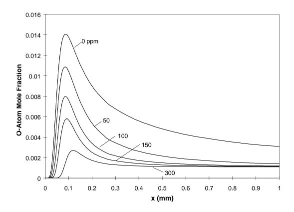
Figure 5: Profiles of O-atom mole fraction at different Fe(CO)<sub>5</sub> concentrations.  $\phi$ =1.0,  $X_{O_2ox}$ =0.21,  $X_{H_2}$ =0.01. The equilibrium value of  $X_O$  is 0.0014 for the uninhibited flame and 0.0011 for the inhibited flames.
