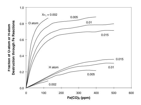
Figure 10: Calculated fractional H-atom and O-atom flux through iron reactions at  $X_{O_2ox} = 0.24$  and varying H<sub>2</sub> concentrations.
