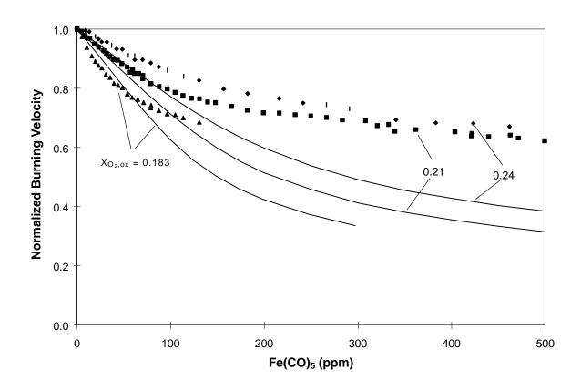
Figure 2: Measured and calculated inhibition effect of Fe(CO)<sub>5</sub> for various O<sub>2</sub> concentrations in stoichiometric CO-H<sub>2</sub>-O<sub>2</sub>-N<sub>2</sub> flames with  $X_{H_2}$ =0.01.
