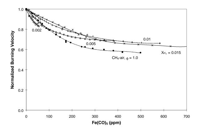
Figure 8: Measured inhibition effect of Fe(CO)<sub>5</sub> for various H<sub>2</sub> mole fractions in CO-H<sub>2</sub>-O<sub>2</sub>-N<sub>2</sub> flames with  $\phi$ =1.0 and  $X_{O_2ox}$  = 0.24. For comparison, the normalized burning velocity profile for a  $\phi$ =1.0,  $X_{O_2ox}$ =0.24 CH<sub>4</sub>-air flame [7] is also shown. The uninhibited burning velocities used for the normalizations are listed in the Table 2. Polynomial curve fits of the data are provided for clarity.
