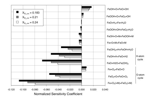
Figure 7: First-order sensitivity coefficients of the burning velocity with respect to reaction rate for selected reactions at  $X_{in}$ = 50ppm, normalized by the peak value for all reactions at all flame locations (which corresponds to CO+OH $\leftrightarrow$ CO<sub>2</sub>+H).
