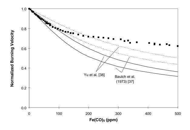
Figure 3: Comparison of experimental data with calculated results using 4 mechanism variations: 2 rates for CO+OH $\leftrightarrow$ CO<sub>2</sub>+H and 2 rates for the catalytic H-atom scavenging cycle. Dotted lines use the slower rates for the reactions in the H-atom cycle; the solid lines, the faster rates.  $\phi$ =1.0,  $X_{O_2,ox}$ =0.21,  $X_{H_2}$ =0.01.
