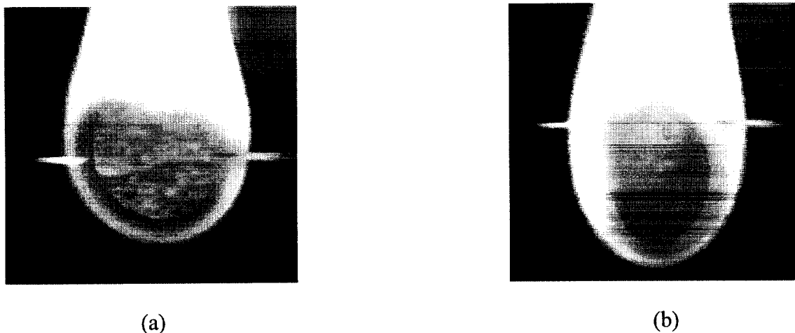
Figure 7. Video images showing a PMMA sphere burning at normal gravity ( D_o = 4.76 mm, 0.10 MPa, and 25 % O_2 ), before (a) and after (b) the occurrence of dripping of the polymer melt.
