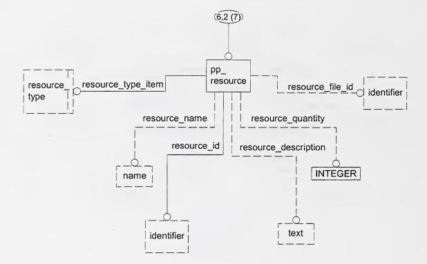
Figure 2.3.7: Process\_Plan\_Operations\_Sheet\_Schema (EXPRESS-G: 7 of 7)
