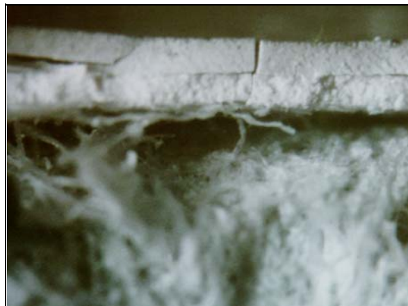
(c) Burned surface near ignition source
